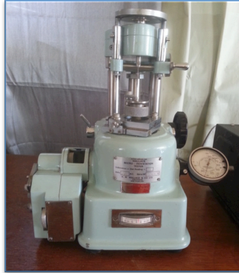
Figure 1-14: Wallace Indenter Microhardness tester.
