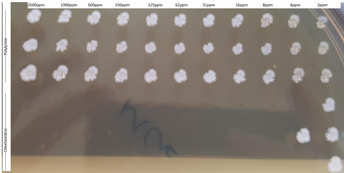
Figure 5-2: Example of an agar plate where the MBC experiment was carried out. Bacteria have grown on the areas where the metal prongs touched the agar after dipping them in the 96 well plate. In this example, the MBC of polylysine is higher than 2000µg/ml and the MBC of chlorhexidine is 8µg/ml.
