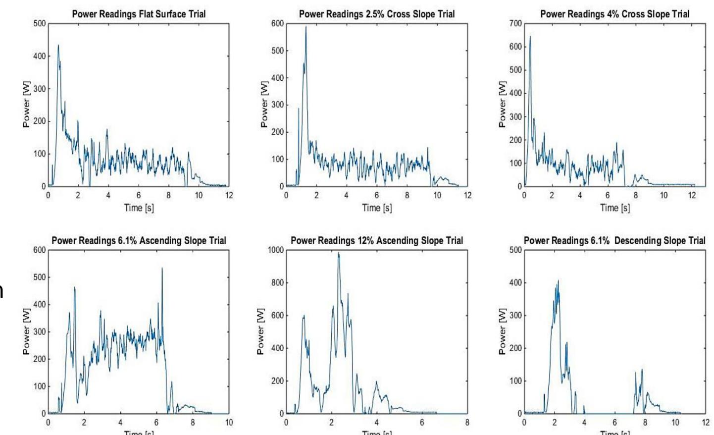
We trimmed power readings to identify three phases of the wheelchair movement: initial acceleration, steady state and stop. An example of a short driving cycle was computed by combining a random series of different microtrips. Conditions included in this representation are flat surface, 2.5% cross slope, 4% cross slope and 6.1% ascending slope
