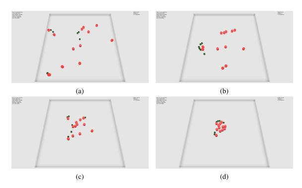
Fig. 5.1 Some snapshots from an example of a swarm of six robots (green cylinders) performing the object (red cylinders) clustering algorithm: a) Initial position of the robots and the objects. b-c) The robots keep pushing the objects to a random location. d) Finally, the robots cluster all the objects in a random location of the arena.
