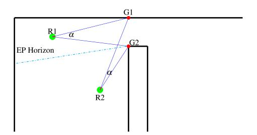
Fig. 5.8 Representation of a section of the environment with two robots pointing to the gap.
