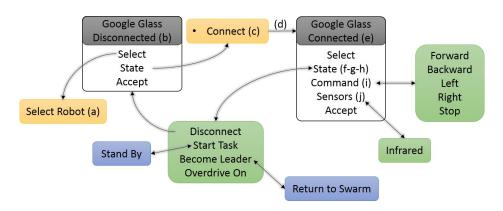
Fig. 3.10 Diagram explaining the architecture of the Google Glass software. The letters next to the instructions and arrows make refference to the screenshots presented in Fig. 3.9.
