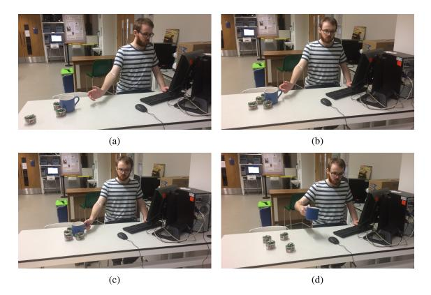
Fig. 2.1 A representation of a human working with a computer while requesting the robots to transport his mug closer with a simple hand gesture. a) The user moves his hand requesting the robots to transport the mug. b) The robots group next to the mug and start pushing it towards the user. c) The user finally grabs the mug. d) The user lifts up the mug and the robots return to their initial position.
