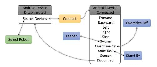
Fig. 3.6 Diagram of the architecture of the Android mobile device software.
