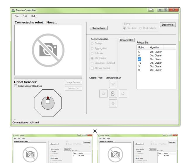
Fig. 5.3 a) GUI with a list showing the IDs of some previously connected robots. b) Example snapshot of the GUI when the sensors' feedback is activated. c) An example with the sensors' feedback activated and the raw data visible.
