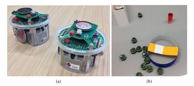
Fig. 3.1 (a) The real e-puck robot. (b) A group of e-puck robots pushing the object towards the (red robot) dynamic goal.
