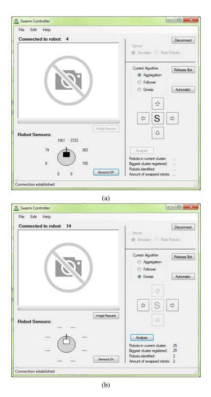
Fig. 4.7 a) The GUI presenting the IR sensor readings from the leader robot. b) The GUI presenting the unit count of the local cluster from the leader robot perspective.
