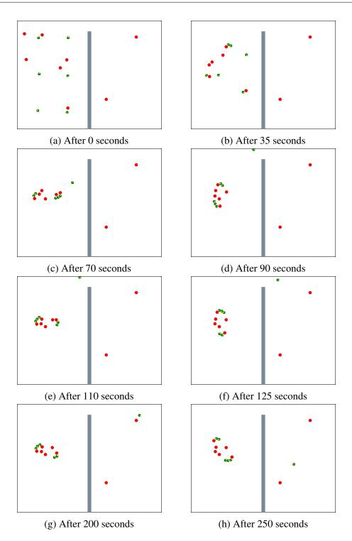
Fig. 5.14 Sequence of snapshots taken during a trial of a participant from group "C". The red dots represent the objects, the green dots represent the robots and the middle wall is represented by the gray line in the middle.
