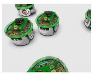
Fig. 4.1 The e-puck miniature mobile robot in the simulation.
