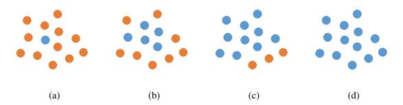
Fig. 4.4 The gossip algorithm relays a command to the nearest neighbours. a) The leader robot receives a new command from the operator. b) It relays it to the nearby robots. c) The nearby robots relay the message to their locally connected robots. d) Finally all robots have relayed the message to all the locally connected robots.
