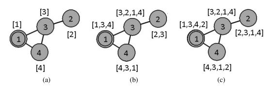
Fig. B.1 Example of robots counting (lines denote pairs of robots within communication range). (a) Initially, only their own ID is in the list. (b) The robots include the IDs received by their neighbors. (c) After a further iteration, each robot contains everyones' IDs in their list. Note that perfect communication is assumed. In practice, the e-pucks may be unable to receive multiple messages simultaneously.
