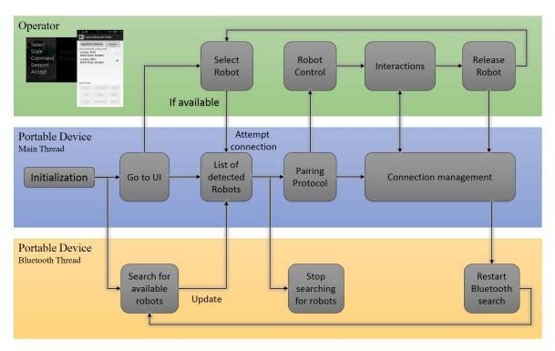
Fig. 3.3 User interface software architecture representation.
