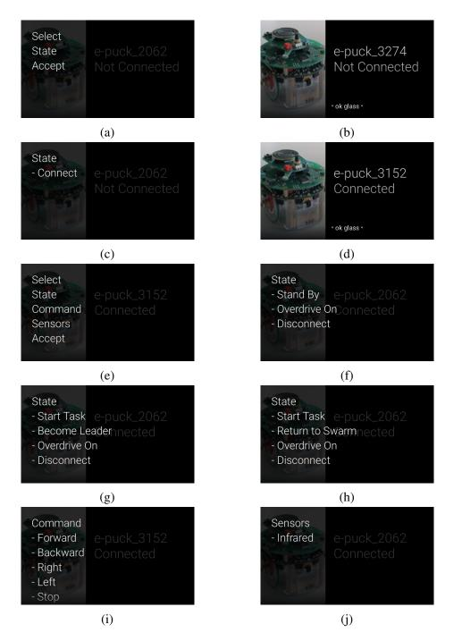
Fig. 3.9 Snapshots taken from the Google Glass interface: a) Disconnected "Main" menu. b) Disconnected Selection list. c) Disconnected "State" menu. d) Connected list. e) Connected "Main" menu f) Connected "State" menu while active. g) Connected "State" menu during "Stand-By" as swarm unit. h) Connected "State" menu menu during "Stand-By" as leader. i) "Commands" menu. j) "Sensor" menu .
