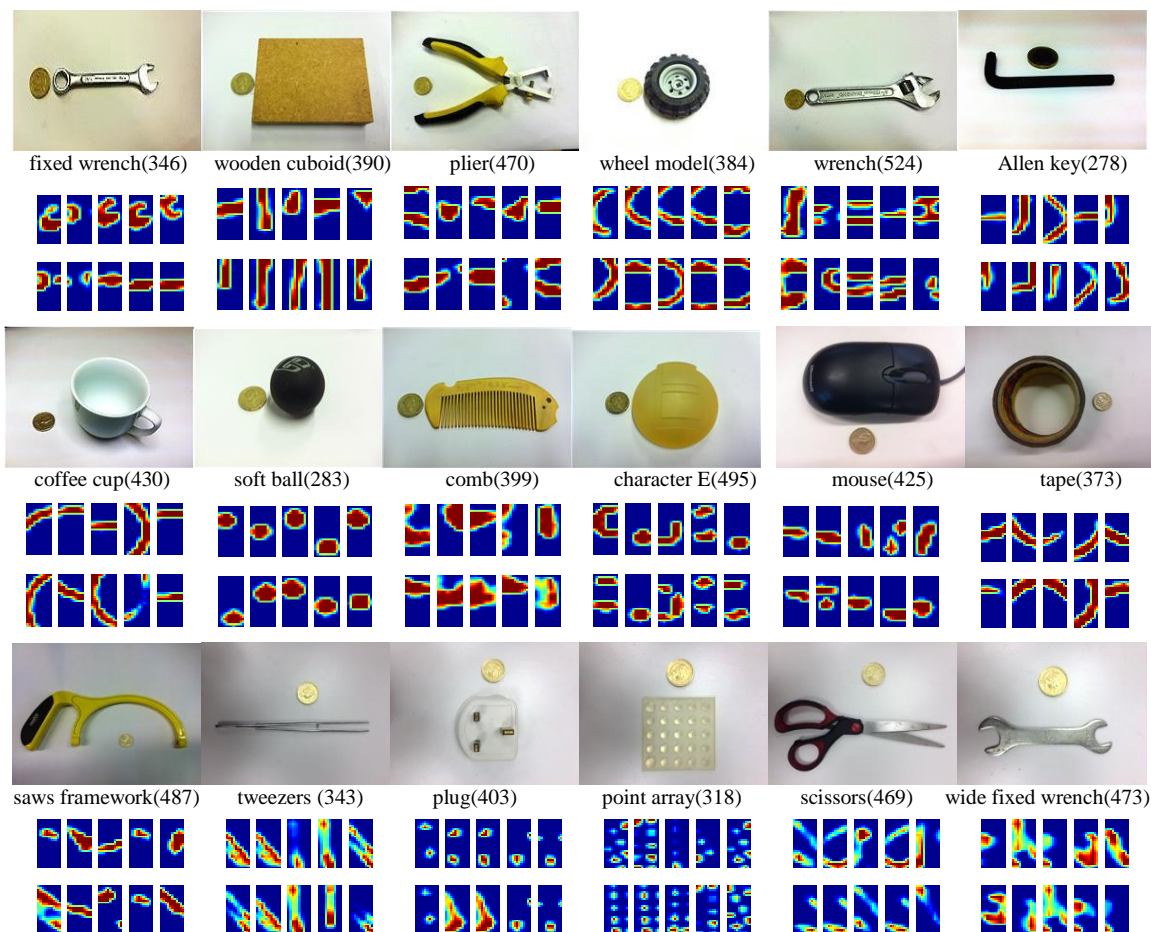
Fig. 6. Objects used for tests. First, third and fifth rows are visual images of objects. The name and number of collected tactile readings are also listed under the picture of each object. Second, fourth and last rows are corresponding sampled tactile images, in which prominent features can be observed.
