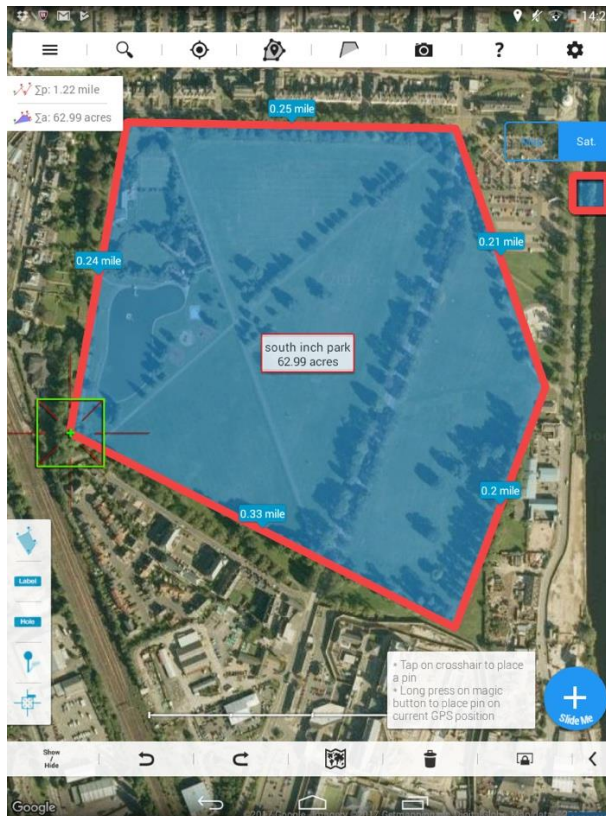
Figure 4-3. Screenshot of the application Measure Map showing area and perimeter of enclosed space.
