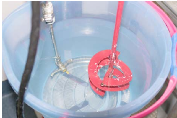
(B) Details of the mixer blade (right) with ADV head on the left
