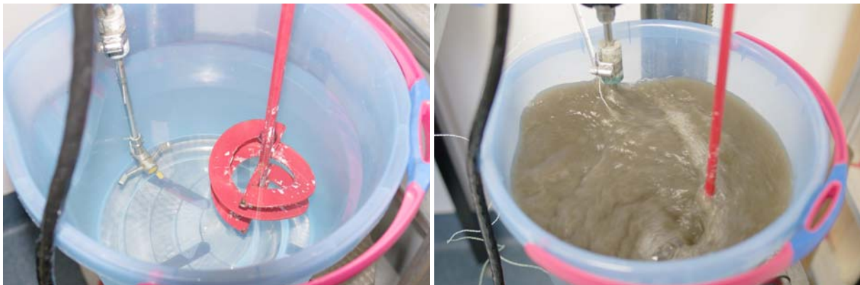
(B, Left) Details of the mixer blade (right) with ADV head on the left (no water)
