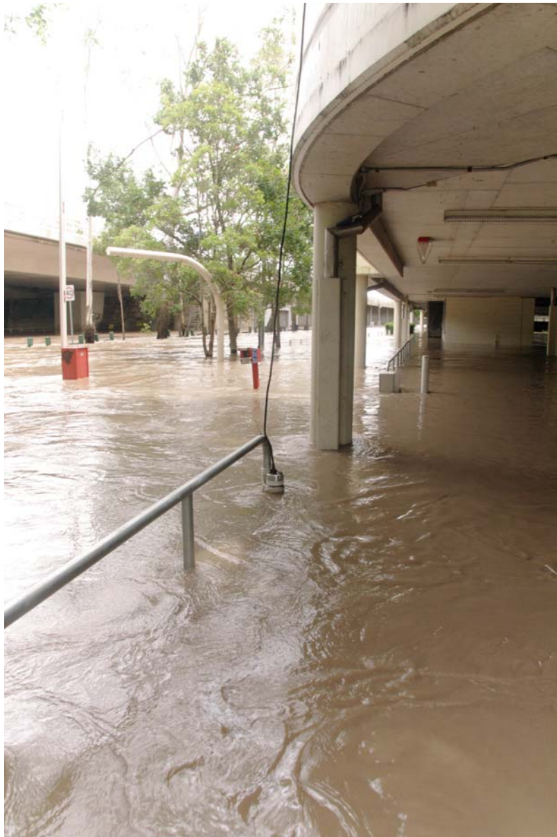
Fig. A-11 - View of the boom gate pylon and the handrail supporting the ADV system on Thursday 13 Jan. 2011 at 11:39 (Photograph Hubert CHANSON) - Pentax™ K-7 with Pentax™ DA18-250mm f3.5-6.3 ED AL lens - Flow from background right to left
