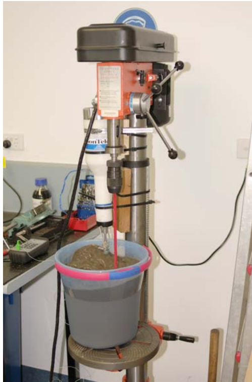
(A) Test for SSC = 70.5 \text{ kg/m}^3 - The ADV system is in the background with the water mixers slightly in the right
