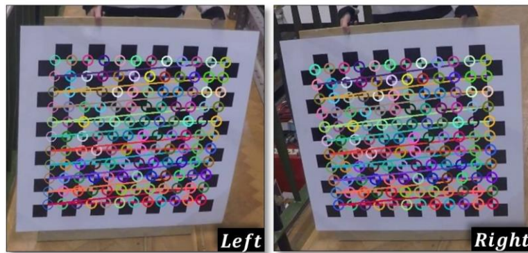
Figure 4-18: Detection of corresponding points for stereo camera calibration.
