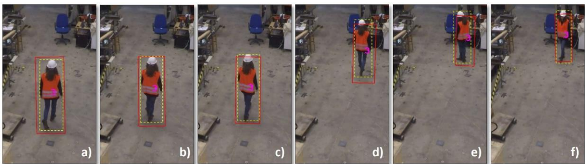
Figure 4-13: Drifting issue of a computer vision tracking method under walking (a-d) and posture variations (e-f).
