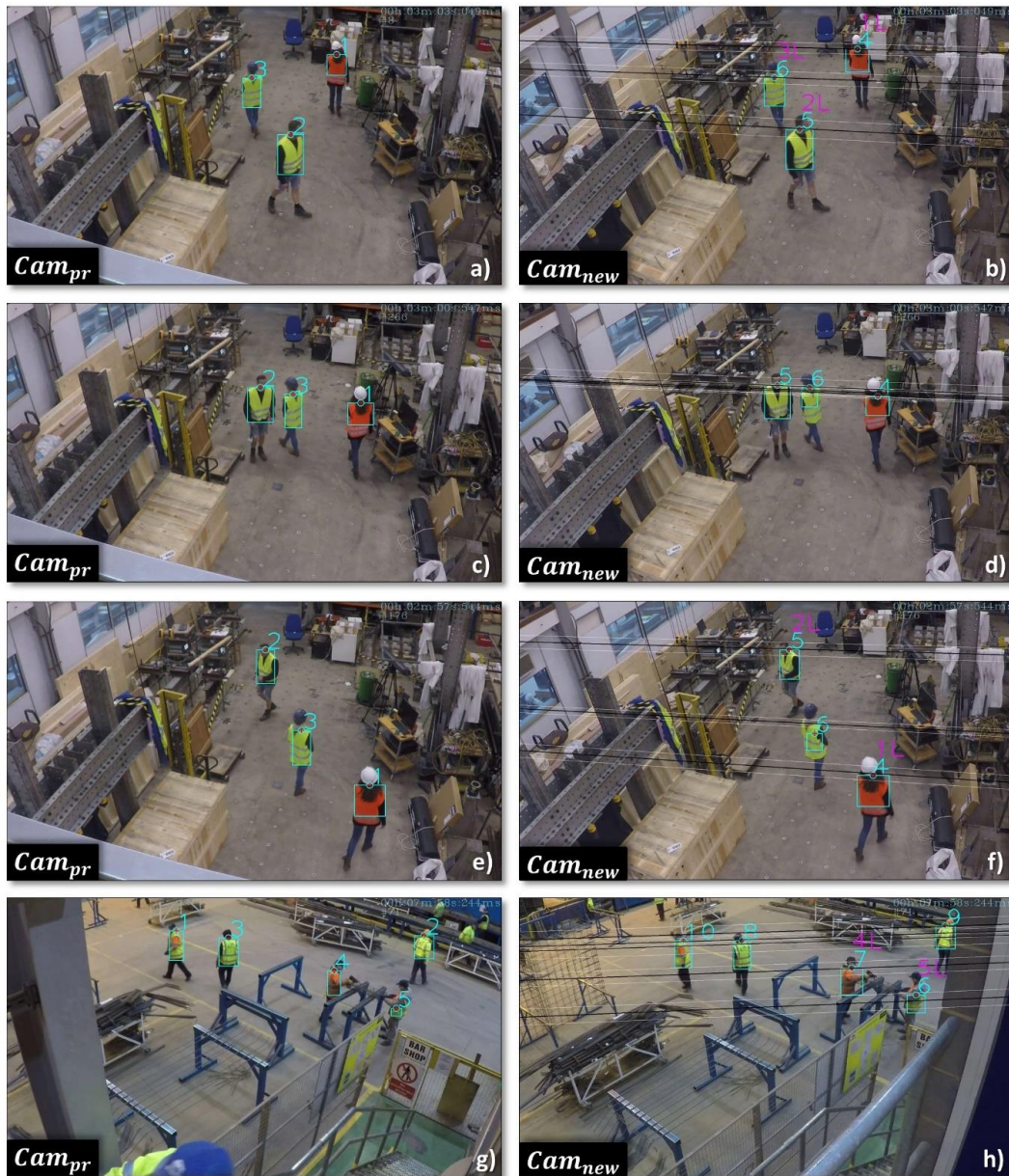
Figure 4-25: Performance examples of the geometry-based matching method. (a-b) Three TP matches, (c-d). Three TN matches due to congestion. (e-f) Two TP matches and one FN caused by tracking inaccuracy (Data set A). (g-h) Three TN matches due to congestion and two TP (Data set B).
