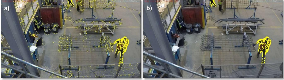
Figure 3-11: Example of frame differencing between successive frames for motion extraction. (a) Noisy outcome. (b) Denoised outcome.
