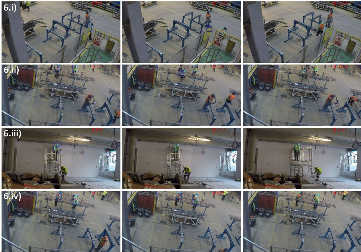
Figure 3-25: Screenshots of the performance of the proposed tracking method (cyan coloured rectangle) and Park2016 (dark blue coloured rectangle) under almost total occlusions (worker in 6.i, worker “0-2” with orange Hi-Vis in 6.ii, and worker in 6.iii) or by partial occlusions (worker “1-3” with yellow Hi-Vis in 6.ii, and both workers in 6.iv).
