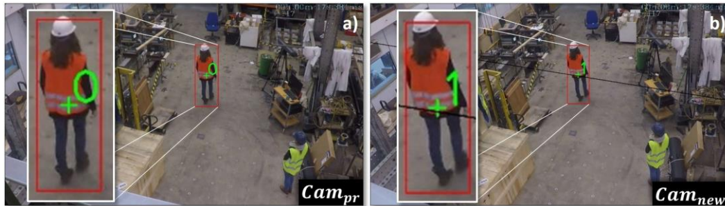
Figure 4-12: False negative (FN) matching of a single worker between two cameras (a-b).
