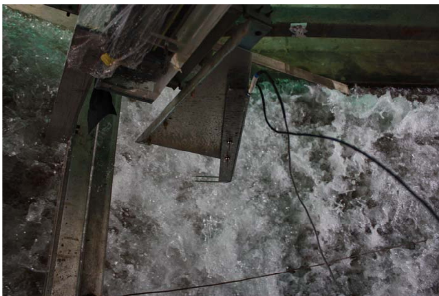
Fig. 3 - Experimental setup with two single-tip conductivity probes side-by-side - Flow from left to right
