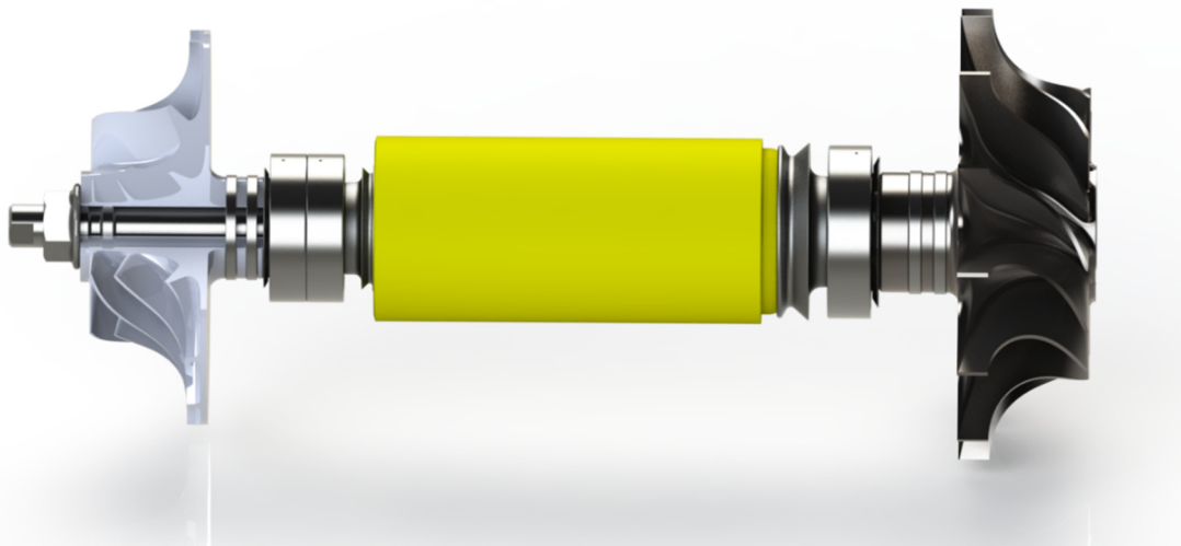
Figure 3.9: MGT shaft arrangement
