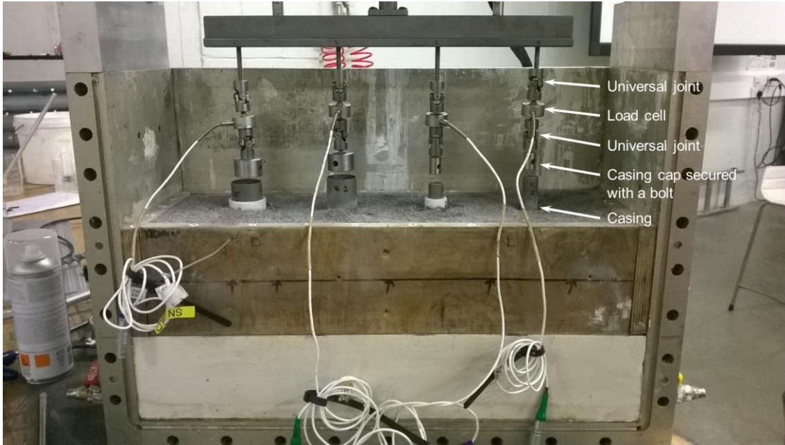
Figure 3. Casing and connector components set up used in Test 5
