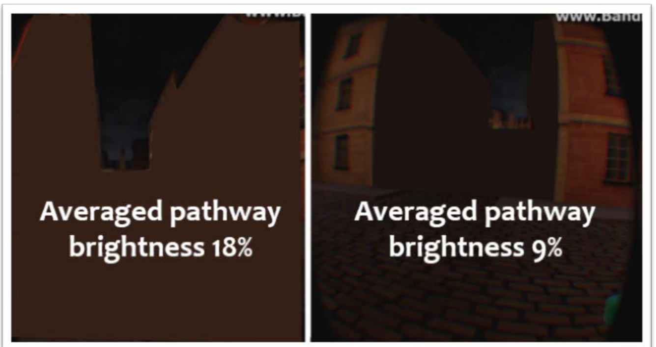
Figure 180. An example of the screen area averaging method used to determine the overall brightness of a path in the VR version of the apparatus. The dark path [right] was only 50% as bright as the bright path [left].
