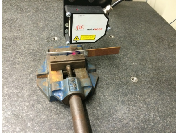
Fig. 3: Laser scanner used for surface profiling of friction stir welded Al and Cu samples.
