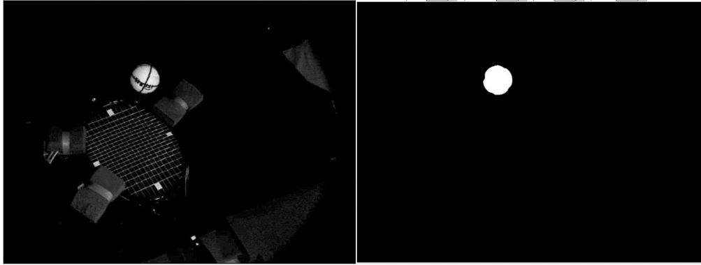
Figure 6.4 – Example images of an impact test with ball in shot: unprocessed (left) and processed (right) to leave only the ball.
