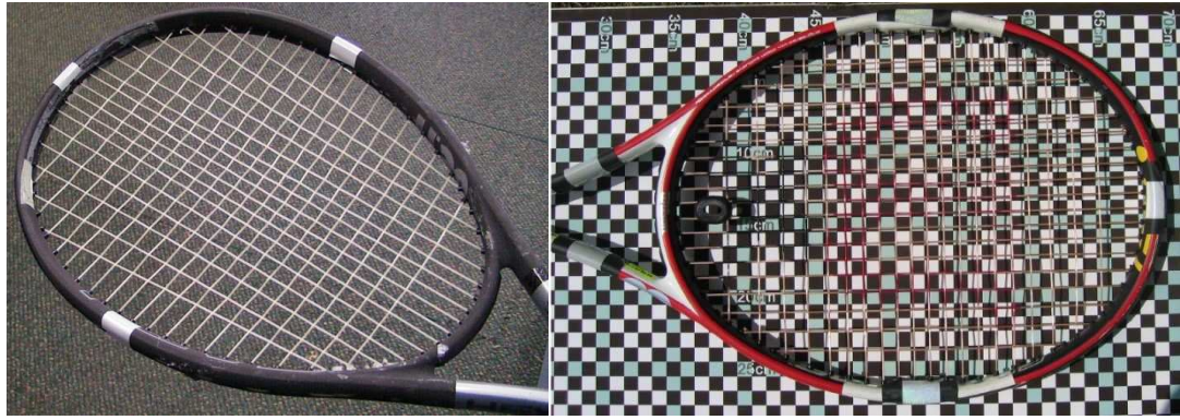
Figure 2.20 – Choppin (2009) measured impact locations using reflective tape attached to the racket frame as reference points (left). The positions of the reflective tape relative to the geometric stringbed centre were established from a racket calibration image (right).
