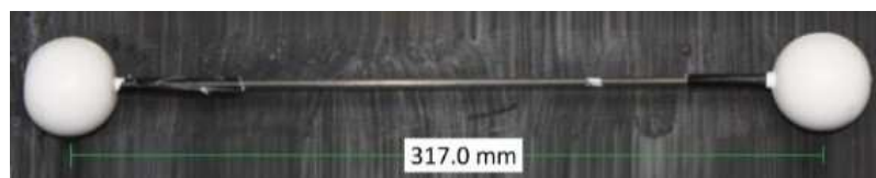
Figure 4.2 – The calibration object comprised two squash balls coated in white paint attached to both end of a plastic rod. The distance between the squash ball centres was 317.0 mm.
