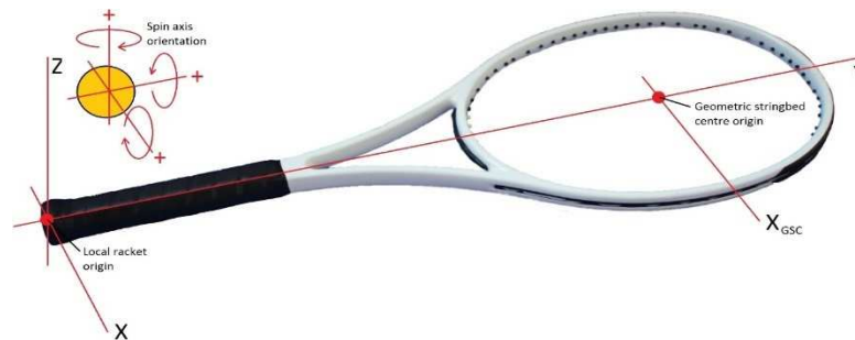
Figure 10.2 – Local racket origin for transformed ball velocity, ball spin axis and impact location measurements. The longitudinal component of impact locations were translated to the geometric stringbed centre.
