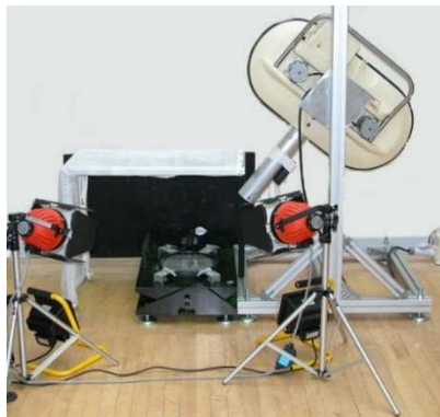
Figure 3.2 – The Spin Rig was the basis for the Impact Rig. The Spin Rig used a BOLA ball launch device to launch a ball with variable inbound velocity and spin onto a head-clamped racket.
