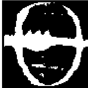
Figure 2.17 – The SpinTrack3D algorithm inverted the colour of the segmented ball markings resulting in a closely cropped binary image.
