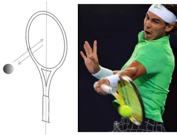
Figure 2.7 – The ball-racket impact model is limited to normal impacts along the longitudinal axis of the racket (left). Real tennis impacts can be oblique, off-axis and include spin (right).
