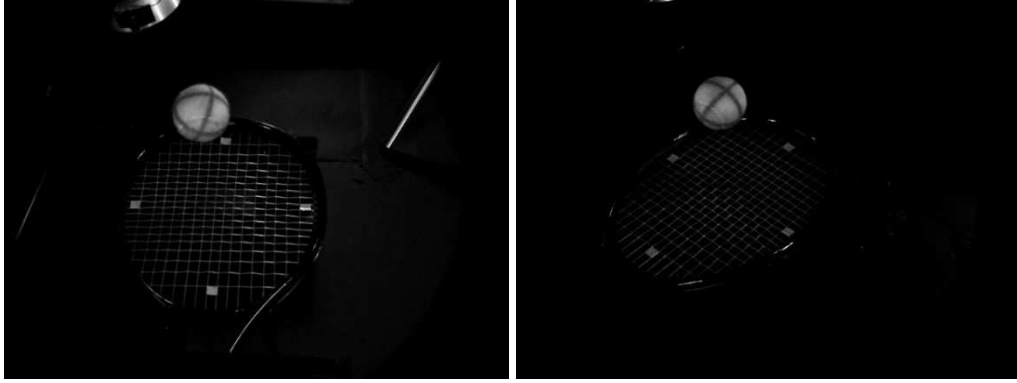
Figure 6.13 – Example images of the ball during an impact test imaged in the left (left) and right (right) cameras.
