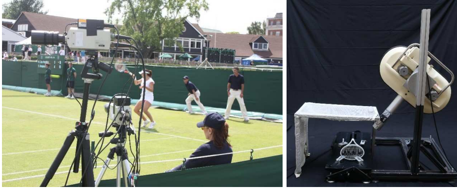
Figure 2.1 – Measuring spin rate during real-play at the Wimbledon Qualifying event (left) and the ITF Racket Spin Rig to measure spin generation of different strings (right).
