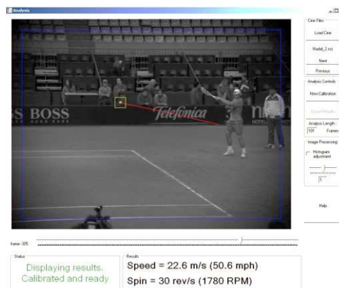
Figure 2.10 – Kelley (2011a) developed a methodology to measure ball velocities and spin rates from single high-speed videogrammetry of real-play in tennis.
