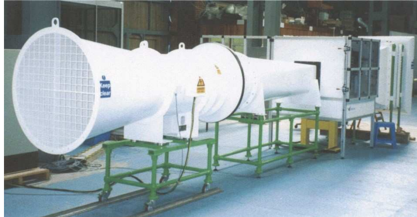
Figure 2.6 – The ITF wind tunnel was used to measure the C_D and C_L for non-spinning and spinning tennis balls.
