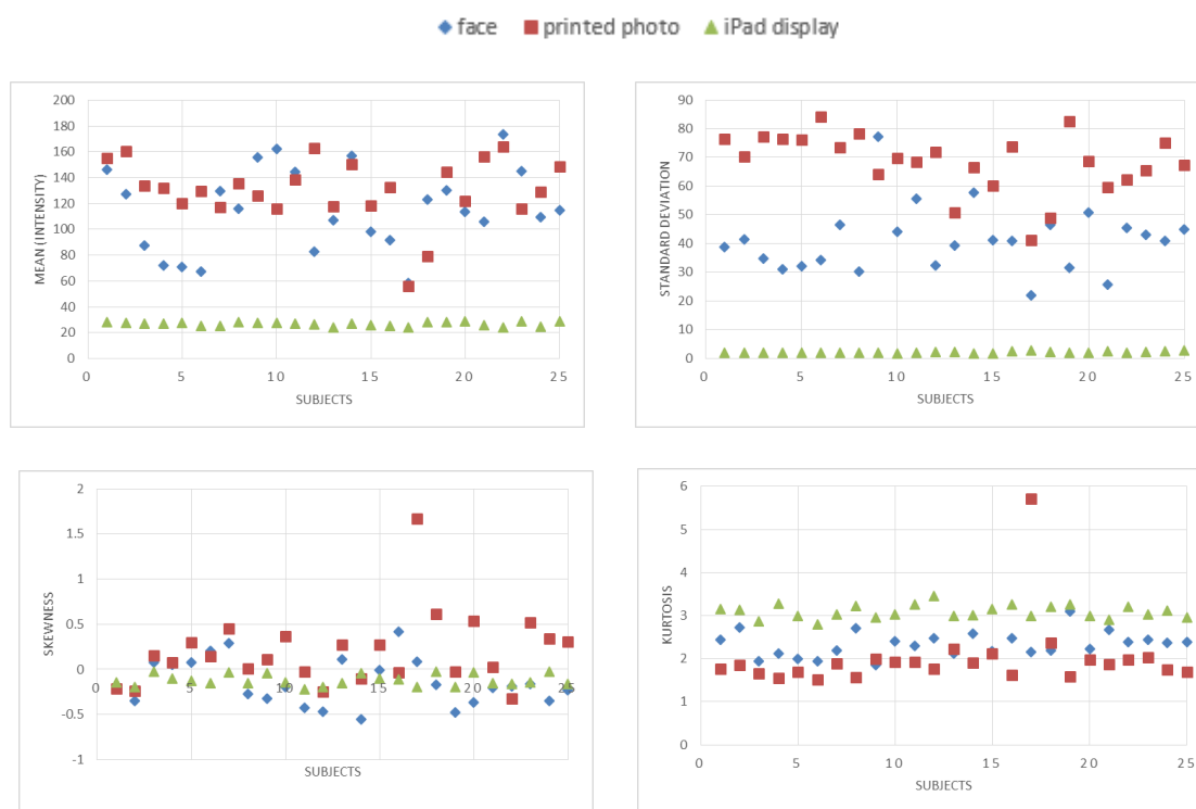
Figure 5.16: Statistical analysis on the NIR Img_{90} images for the real face, printed photo faces and iPad displayed faces
