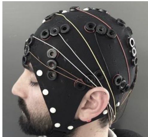
Figure 2 Triplet holders distributed at 10-20 positions held together by a cap. 19 locations arranged according to the International 10-20 System were selected over the whole head.
