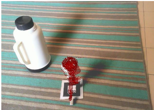
Figure 10 Soft shadows for a Bobo boy with 373544 triangles using QSI
