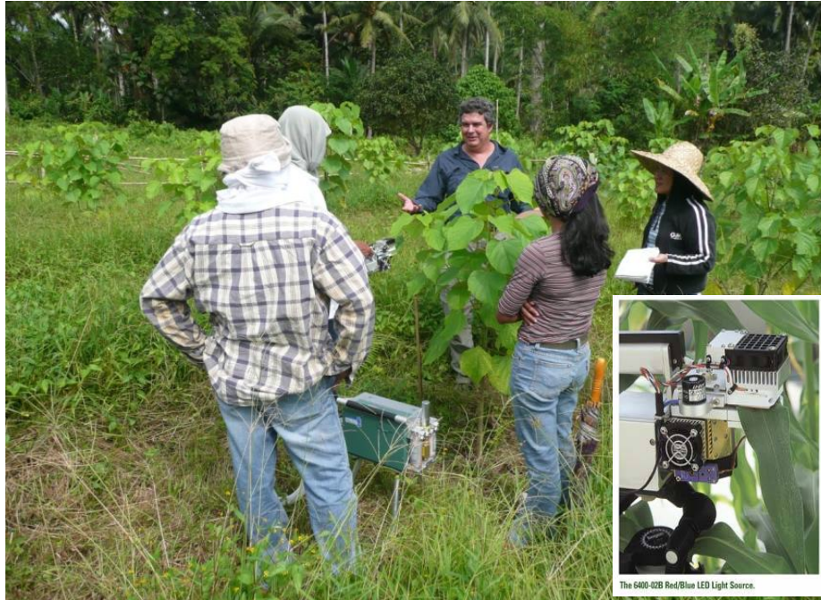
Figure 8. Measurement of photosynthesis in ACIAR field trials using a portable infrared gas analyser
