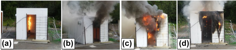
Figure 6. PIR panel enclosure: (a) at ignition; (b) after 8 min; (c) after 11 min; (d) after 24 min.
