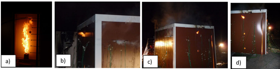
Figure 7. Stone wool panel enclosure: (a) at ignition; (b) after 12 min; (c) after 30 min; (d) after 32 min. (b)–(d) A rear view of the compartment with flaming visible at holes and opened joint.
