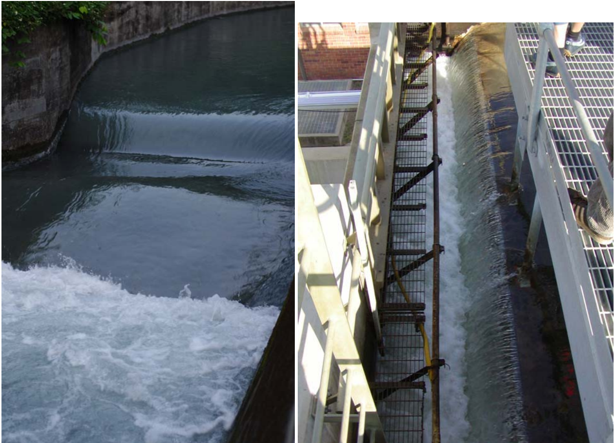
(A, Left) Hydraulic jump in an irrigation channel on 10 May 2010 in Hualien County (Taiwan) - Flow from top right to bottom left (Shutter speed: 1/100 s)
