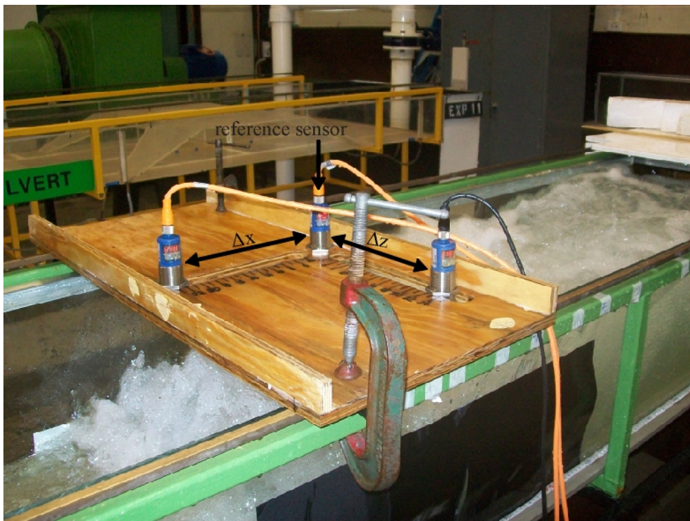
Fig. 2 - Experimental setup with three acoustic displacement meters and definition of the longitudinal and transverse separation distances \Delta x and \Delta z - Flow from left to right: d_1 = 39.5 mm, x_1 = 1.50 m, Fr_1 = 5.1 , Re = 1.3 \times 10^5
