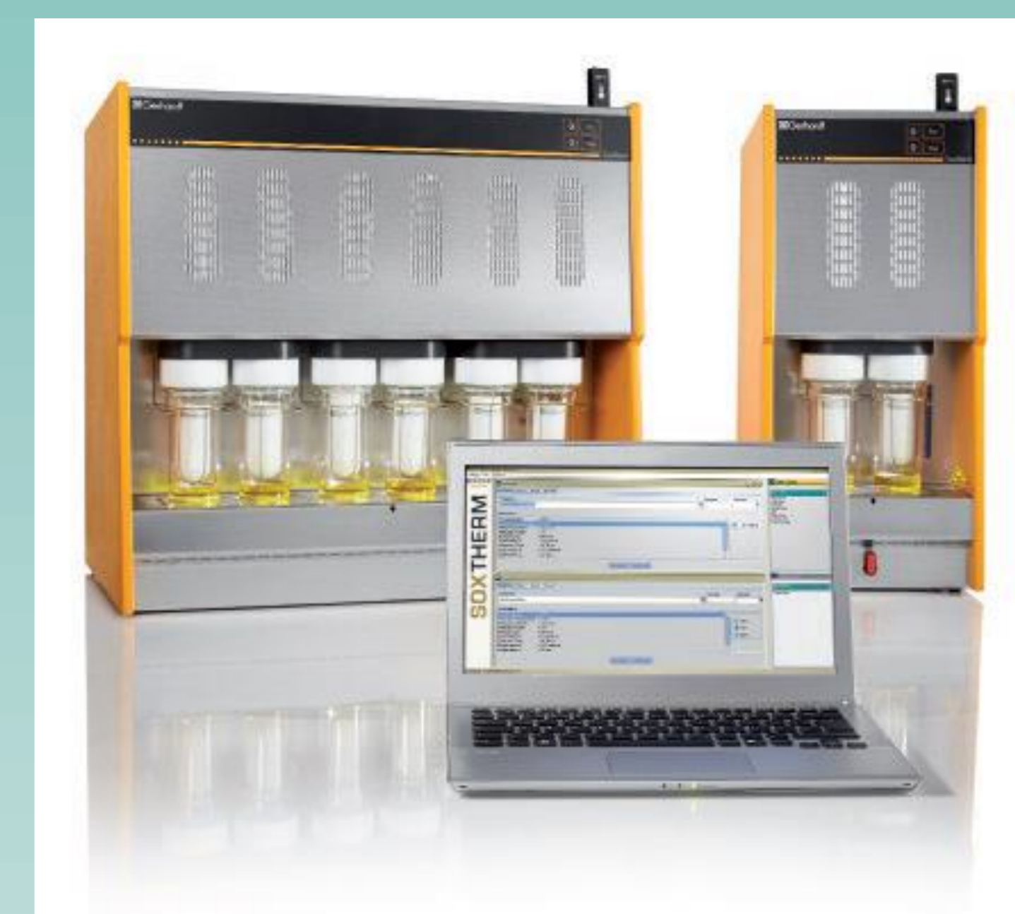
SOXTHERM – rapid extraction system for solid-liquid extractions
