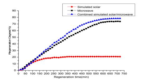
**Figure 7.** Variation of the regeneration degree for the solar solid dehumidification/regeneration bed under the three regeneration methods.
