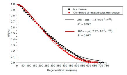
**Figure 12.** Comparison of the moisture ratio from the testing and semi-empirical Page model results [27].
