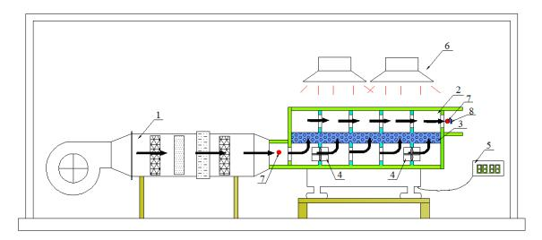
**Figure 2.** The structure of the test rig: 1—DC air conditioner; 2—solar solid dehumidification/ regeneration bed; 3—silica gel; 4—microwave generator; 5—electronic scale, 6—xenon lamps, 7—temperature/humidity sensor, 8—Pitot tube anemometer.
