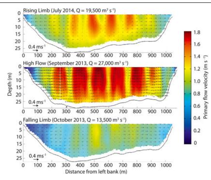
**Figure 3.** Primary flow velocities with secondary flow vectors for each of the three surveys conducted at the bifurcation head (XS001; Figure 1A). Data were collected using a 600 kHz aDcp. The vertical 'stripes' evident in the data represent the presence of bridge piers located ~200 m upstream of the survey line. [Colour figure can be viewed at wileyonlinelibrary.com]
