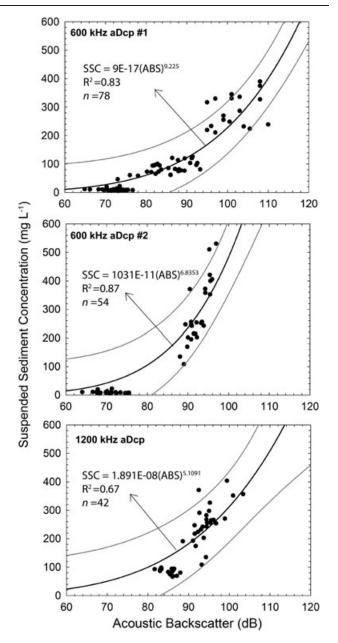
**Figure 2.** Relationships between corrected acoustic backscatter (dB) and measured suspended sediment concentration (mg L<sup>-1</sup>) for the three aDcp units used in the study. 95% prediction bounds are shown in grey. For all fits, *P* < 0.05.
