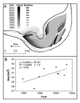
**Figure 8.** (A) Island areal extents and banklines determined from Landsat imagery over the period 1959–2013. (B) Total area covered by the island complex as a function of year calculated from the areas masked in the Landsat imagery depicted in panel (A), showing average annual aggradation/progradation of 0.05 km<sup>2</sup> a year.
