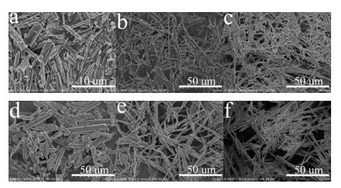
Fig. 1 SEM images of the samples prepared in different solutions at 90 °C. CaCl<sub>2</sub> aqueous solution and KPS aqueous solution (a), KPS EG solution (b) and KPS GL solution (c); CaCl<sub>2</sub> and KPS DMF solutions (d), KPS EG solution (e) and GL solution (f).
