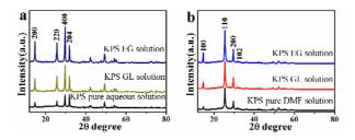
Fig. 2 XRD patterns of the whiskers prepared in different solutions at 90 oC. (a) aqueous solution; (b) DMF solution.
