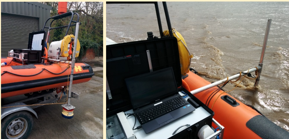
Figure 2 Mounting the Teledyne Workhorse ADCP
