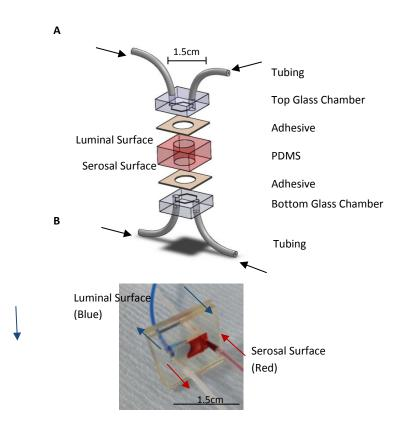
Fig 1: The dual flow device. Panel A: Schematic of the dual flow device used to hold human gut tissue in a known orientation. Panel B: Coloured food dye depicting the dual flow in the microfluidic device.
