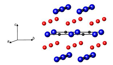
**Figure 9.** Representation of CaNiN. The red, black, and blue spheres represent calcium, nickel, and nitrogen, respectively.
