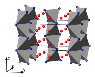
**Figure 2.** Representation of Li<sub>3</sub>FeN<sub>2</sub>. The red and blue spheres represent lithium and nitrogen, respectively. The chains of grey polyhedra represent the  $\frac{1}{\infty}$ [FeN<sub>4/2</sub><sup>3-</sup>] chains.
