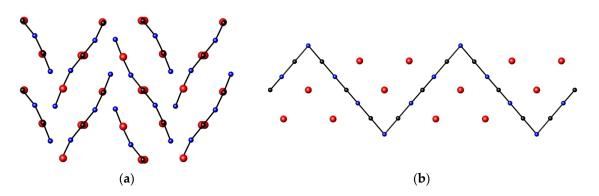
**Figure 10.** Representation of SrNiN showing (**a**) the herringbone stacking, viewed along [010] and (**b**) the zigzagging chains, viewed along [100]. The red, blue, and black spheres represent strontium, nitrogen, and nickel atoms, respectively.
