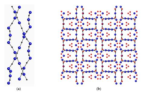
**Figure 12.** Representation of  $Ba_8[(NiN)_6]N$ . (a) Shows the intertwining  $\frac{1}{\infty}[NiN_{2/2}^{2-}]$  chains (for clarity barium has been omitted) and (b) shows  $Ba_8[(NiN)_6]N$ , viewed along [001]. The red, blue, and black spheres represent barium, nitrogen, and nickel, respectively.
