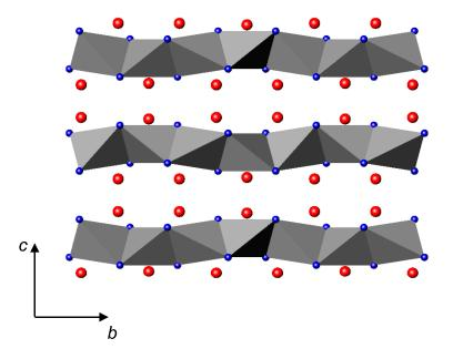
**Figure 3.** Representation of  $Ba_3Ga_2N_4$ . The red and blue spheres represent barium and nitrogen, respectively. The chains of grey polyhedra represent the  $\frac{1}{\infty}[GaN_{4/2}^{3-}]$  chains.
