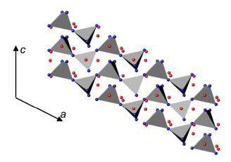
**Figure 4.** Representation of Na<sub>3</sub>MN<sub>3</sub>, M = W, Mo. The red and blue spheres represent sodium and nitrogen, respectively. The chains of grey polyhedra represent the  $\frac{1}{\infty}[MN_{4/2}^{3-}]$  chains.
