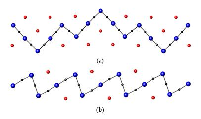
**Figure 11.** Representations of the chains in (**a**) BaCoN and (**b**) BaCuN. The red, black, and blue spheres represent barium, cobalt/copper, and nitrogen, respectively.
