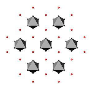
**Figure 1.** Representation of NaBa<sub>3</sub>N viewed along [001]. The red and black spheres are sodium and barium, respectively. The grey polyhedra are  $Ba_6N$ .
