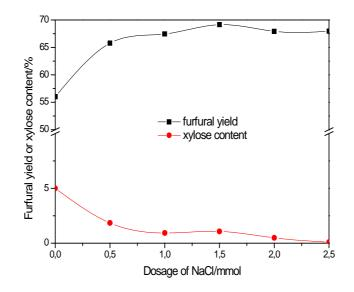
**Figure 5.** Effect of NaCl addition on the furfural yield and xylose contents. Reaction conditions: D-xylose (1.0 mmol), SSP (10 wt%), water (1 mL), CPME (3 mL), MW, 190 °C, 40 min.
