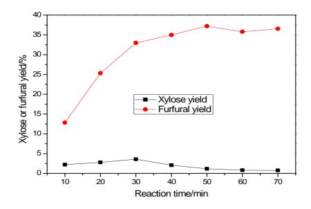
**Figure 8.** Furfural yield and xylose contents from xylan against reaction time. Reaction conditions: xylan (1 mmol based on xylose units), SSP (10 wt%), NaCl (1,5 mmol), water (1 mL), CPME (3 mL), MW, 190 °C.
