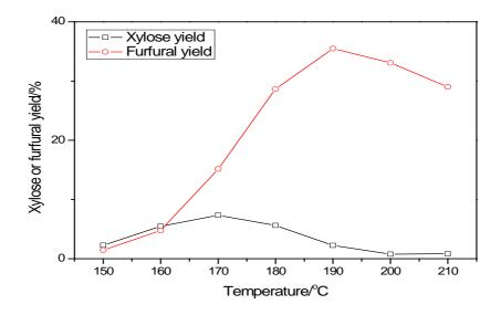
**Figure 7.** Furfural yield and D-xylose contents from xylan against temperature. Reaction conditions: xylan (1 mmol based on D-xylose units), SSP (10 wt%), NaCl (1.5 mmol), water (1 mL), CPME (3 mL), MW, 40 min.
