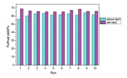
**Figure 6.** Reusability of the catalyst. Reaction conditions: D-xylose (1.0 mmol), SSP (10 wt%), NaCl (1.5 mmol), water (1 mL), CPME (3 mL), MW, 190 °C, 40 min.
