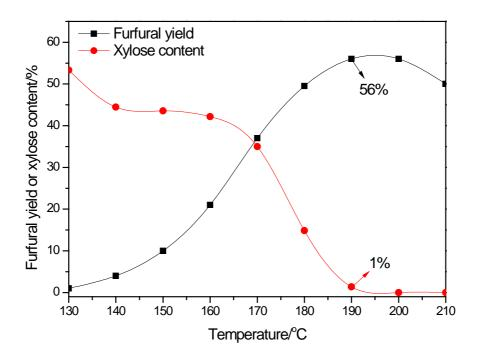
**Figure 1.** Effect of temperature on the yield of furfural and D-xylose content. Reaction conditions: SSP (10 wt%), D-xylose (1.0 mmol), water (1 mL), CPME (3 mL), MW, 60 min.
