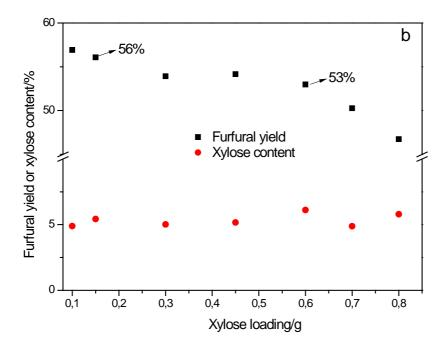
**Figure 4.** D-Xylose loading on the yield of furfural and xylose contents. Reaction conditions: SSP (10 wt%), water (1 mL), CPME (3 mL), MW, 190 °C, 40 min.
