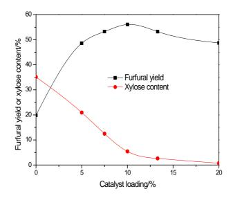
**Figure 3.** SSP catalyst loading on the yield of furfural and xylose contents. Reaction conditions: D-xylose (1.0 mmol), water (1 mL), CPME (3 mL), MW, 190 °C, 40 min.
