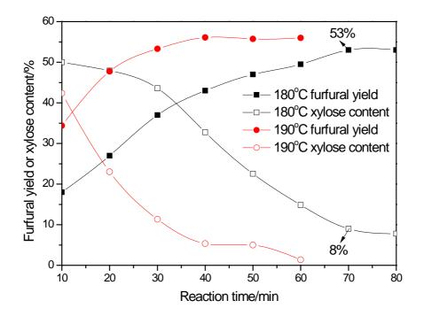
**Figure 2.** Effect of reaction time on the yield of furfural and D-xylose contents. Reaction conditions: SSP (10 wt%), D-xylose (1.0 mmol), water (1 mL), CPME (3 mL), MW, 190 °C.
