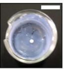
Fusing the dry supra-particle at 106 °C for 2 hours
