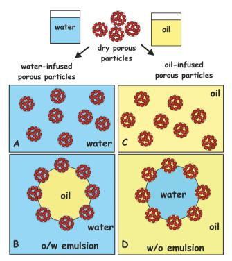
Scheme 3 Effect of the pre-infusion of the porous particles with water (A) and oil (C) on the favoured type of Pickering emulsion obtained upon using the pre-infused porous particles as emulsifiers: (B) oil-in-water emulsion and (D) water-in-oil emulsion.
