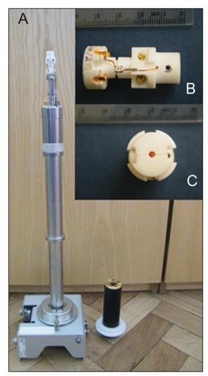
**Fig. 2** (A) Photograph of the probe used for the MRI experiment to visualise the penetration of liquid into the porous particles. Insets show side (B) and top (C) photographs of the solenoid coil which is attached to the top of the Bruker microimaging probe shown in (A).
