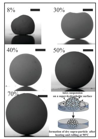
**Fig. 3** Optical images of supra-particles formed by evaporation of sulphate latex suspension of various particle concentrations (8–70 wt%, shown) on a super-hydrophobic surface at 90 °C. The latex suspension drop was rolled over the hot super-hydrophobic surface until complete evaporation occurred. All scale bars are 0.50 mm.
