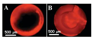
**Fig. 9** Fluorescence microscopy images of a porous supra-particle impregnated with  $10^{-5}$  M Rhodamine 6G solution after (A) 1 hour and (B) overnight. The particles were fragmented after infusion with the liquid before being observed and imaged on a fluorescence microscope using a TRITC filter set. Particles were obtained from a 40 wt% latex suspension (see Table 1 for more details).
