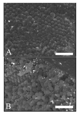
**Fig. 10** SEM images represent the infusion of an aqueous solution of silver nitrate inside the pores of a supra-particle; (A) is a SEM image of the supra-particle's outer surface, while (B) is a SEM image of the inner structure at the edge of a fractured supra-particle. The particles were removed from the solution and dried up before imaging. Silver nitrate nanocrystals appear as bright spots on the images. The scale bars are 10 μm.
