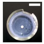
Rolling the latex suspension on a hot super-hydrophobic surface
