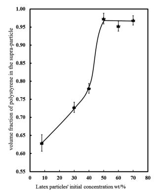
**Fig. 8** Relation between the latex particles' initial concentration in w/w% (*x*-axis) and the volume fraction of sulphate latex particles in the supraparticles (*y*-axis). The volume fraction of these particles increased with the increase in the particles' initial concentration and reduced the pore fraction of the total particles. Above 50 wt%, the latex particle volume fraction levelled off.
