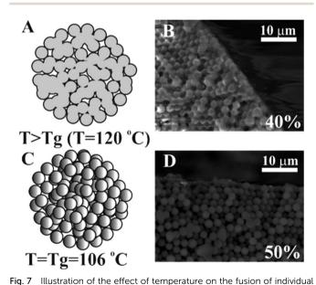
polystyrene latex particles inside a composite supra-particle: (A) a diagram of the fusion of latex particles annealed at  $T > T_g$ ; (B) a SEM image of a supra-particle made from a 40 wt% latex particle suspension annealed at 120 °C; (C) a diagram of a supra-particle annealed at the glass transition temperature ( $T_g$ ) of polystyrene (106 °C); (D) a SEM image of a fractured porous supra-particle made from 50 wt% particle suspension after annealing at  $T_g$ .
