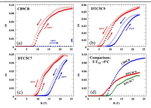
FIG. 3. Effective birefringence measurements as the function of magnetic field B: (a) CB9CB at 130 and 140 °C; (b) DTC5C9 at 169 and 172 °C; and (c) DTC5C7 at 165 and 169 °C. The arrows  $\uparrow(\downarrow)$  show measurements at the field ramping up (down) at a 5 °C/ min rate. (d) Comparison of the three materials at 5 °C above the zero-field  $T_{N-I}$ .
