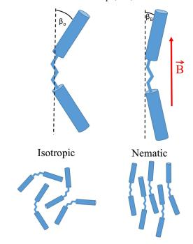
FIG. 4. Illustration of the magnetic-field-induced decrease of the molecular bend, and its consequence of the shift of  $T_{N-I}$ .
