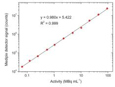
Fig. 2 Plot showing the linearity of the positron detection signal with varying radioactivity levels of the <sup>68</sup>Ga-citrate radiotracer on a log scale.
