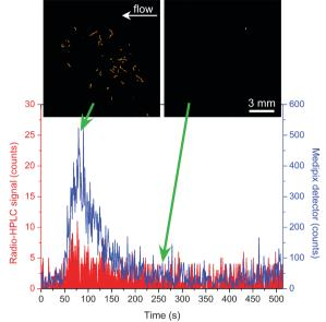
Fig. 3 Plot of  $^{68}$ Ga-citrate radioactive emissions as it passed through the monolithic column. The blue signal shows the signal from the positron detector below the monolith, while the red signal was taken from a flow-through Nal/PMT radio-HPLC detector. Note that the plots are on different scales. Inset are images (14  $\times$  14 mm²) taken from the detector at different time points.
