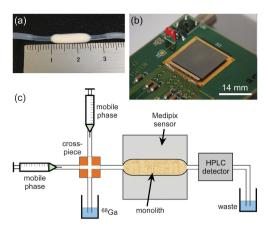
Fig. 1 (a) Silica-based monolithic column encased in heat-shrink tubing. (b) Medipix positron detector, featuring a  $14 \times 14 \text{ mm}^2$  sensor area. (c) Schematic of the experimental setup, with the monolith placed above the Medipix sensor, and featuring a cross-injection system and a standard sodium iodide radio-HLPC detector.
