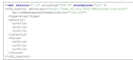
**Listing 9:** An XML document representing a control structure of type stop as defined by the XSD in listing 6 and produced by the program in listing 11. Note that the gravity and force attributes may or may not be used in the shutdown process but the definition of the control structure in listing 6 requires their appearance in the XML document.
