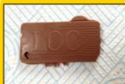
Finished lab-on-a-chip removed from mould
