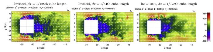
Figure 15. Flow past a cube, comparison of inviscid simulation at resolution 1/128 per cube length and 1/64 per cube length, and with viscous simulation with Re = 1000 at the higher resolution.
