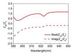
Fig. 3. The real and imaginary parts of the effective impedance of the ZIM.
