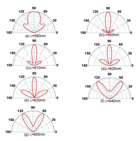
Fig. 5. Calculated emission profile for a plane wave source placed in the middle of the ZIM at center wavelengths of (a)590nm (b)600nm (c)610nm (d)620nm (e)630nm (f)640nm (g)650nm.
