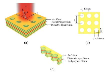
Fig. 1. (a) Diagram of the ZIM consisting of a multilayer stack of 11 alternating layers of 35nm thick Au and 30nm thick dielectric layer with an inter-penetrating two dimensional square array of round holes. The structure is suspended in a vacuum. The lattice constant is L=400nm and hole diameter is d=240nm. The light is emitted from a 30nm thick fluorescent polymer layer within the ZIM. (b) Illustration of round holes array lattice. (c) Scheme of the cross section of the structure.
