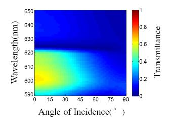
Fig. 4. Simulated angle-and wavelength-dependent transmittance of the ZIM.
