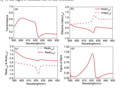
Fig. 2. (a)Theoretical transmittance curves of the ZIM.(b)The real part ( $Real(n_{eff})$ ) and imaginary part ( $Imag(n_{eff})$ ) of the effective refractive index of the ZIM obtained using S-
