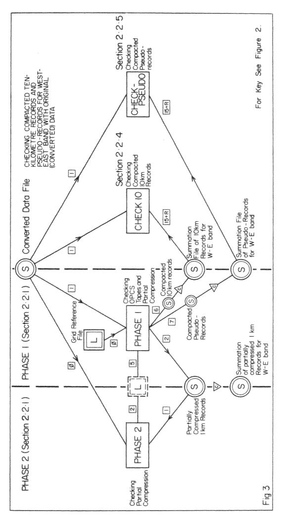
Figure 3: Checking of OPCS tapes and partial compression.
