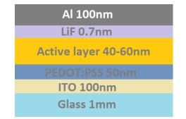
Figure 4 PLED device stack, ITO: Indium-Tin Oxide.
