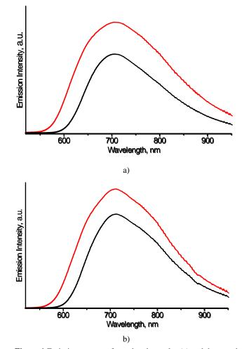
Figure 1 Emission spectra of powdered samples (a) and deaerated dichloromethane solutions (b) of 1 (black line) and 2 (red line).
