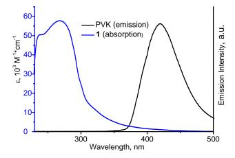
Figure 2 Absorption spectrum of 1 (dichloromethane solution) and emission spectrum of the neat PVK.
