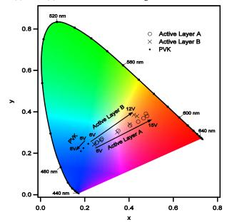
**Figure 7** The colour of the emission of PLEDs with active layer **A** and **B** on the CIE colour diagram. The reference PVK is an identical device fabricated from neat PVK (A and B refer to active layers comprising **A**: 5 mg/ml of  $1^{10}$ @PVK, 2.5 mg/ml of PBD and 1 mg/ml of TPD and **B**: 4 mg/ml of copolymerized cluster  $1^{10}$ @PVK, 2 mg/ml of PBD and 0.8 mg/ml of TPD).
