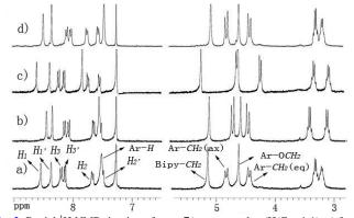
**Fig. 2.** Partial <sup>1</sup>H NMR titration of *cone-*7/guest complex (H/G = 1:1); a) free *cone-*7; b) *cone-*7  $\supset$  Li<sup>+</sup>; c) *cone-*7  $\supset$  Na<sup>+</sup>; d) *cone-*7  $\supset$  Ag<sup>+</sup>; Solvent: CDCl<sub>3</sub>/CD<sub>3</sub>CN (10:1, v/v).
