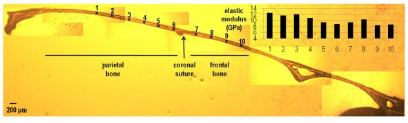
Fig 6. Variation in the elastic modulus of the frontal and parietal bone in the sagittal plane in a P20 WT mouse.
