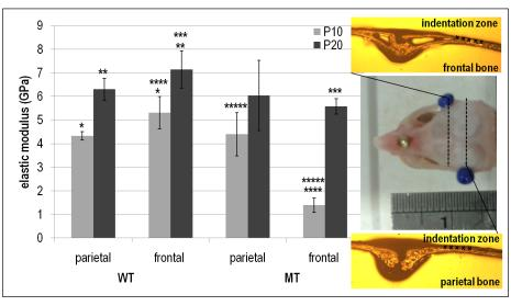
Fig 2. Comparison between elastic modulus of the frontal and parietal bones at P10 and P20 for WT and MT mice. \* highlight statistical significance between corresponding groups (p<0.05).
