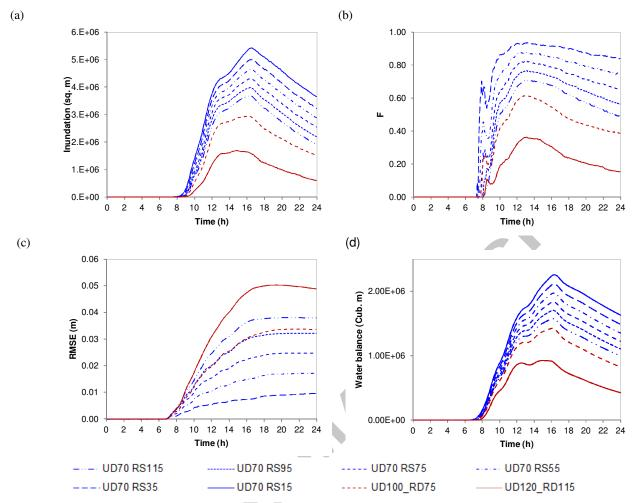
Figure 12: Impacts of improved rural land drainage and storage scenarios through land management: (a) total inundated areas; (b) F statistics compared to the base simulation (UD70/RD15); (c) RMSE compared to the base simulation (UD70/RD15); and (d) water balance for each simulation.
