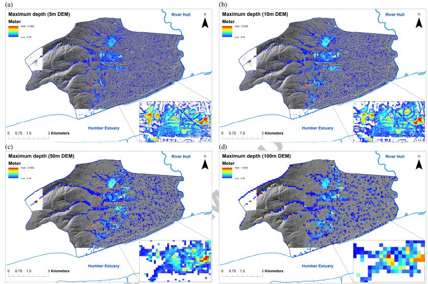
Figure 15: Effects of model resolution: (a) 5 m DTM; (b) 10 m DTM; (c) 50 m DTM, and (d) 100 m DTM.
