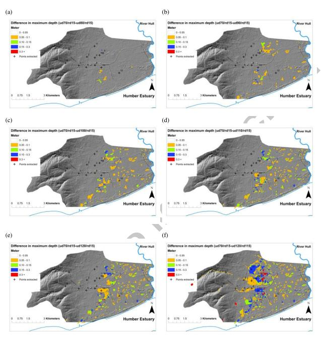
Figure 10: Predicted maximum water depth of the simulations with a 70 mm/day (a) and 120 mm/day (b) urban drainage capacity. Difference in the maximum water depth between the default simulation, and simulations with an improved urban drainage capacity of 120 mm/day (c).
