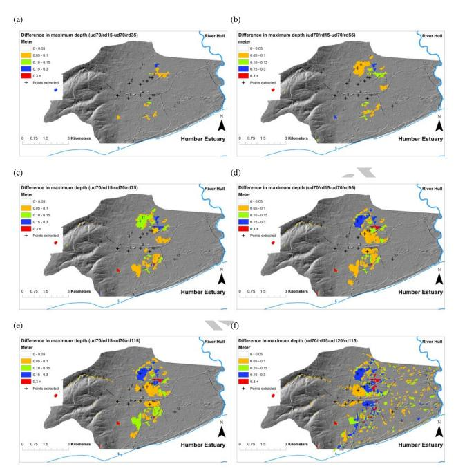
Figure 13: Difference in the maximum water depth predicted between the default simulation and the scenarios with improved rural drainage capacity: (a) 55 mm/day; and (b) 115 mm/day.
