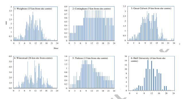
752 Figure 2: Rainfall hyetographs recorded at the gauging stations in and around the city. Unit: mm/15 minutes for sites 1-
