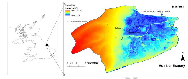
749 Figure 1: Digital Elevation Model of the West part of the City of Kingston upon Hull, UK and contributing catchment
