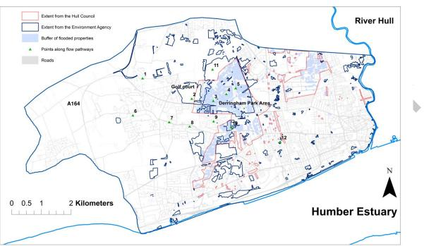
Figure 3: Inundation extent derived from ground survey and aerial photos (UK Environment Agency and Hull City Council); and buffer of properties flooded (Hull City Council).
