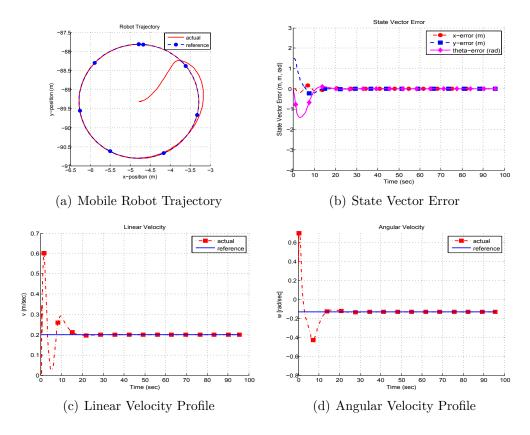
Figure 5.6: Simulation results of trajectory tracking for outdoor navigation
