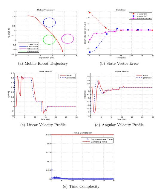
Figure 4.9: Realtime Experimental results of point stabilization with obstacle avoidance
