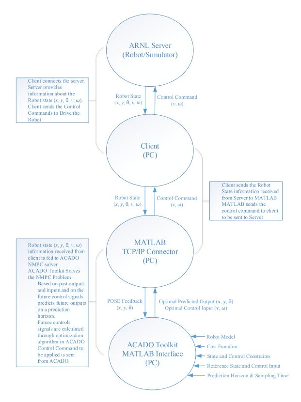
Figure 3.3: Overall Control Strategy for Indoor Navigation using map based localization
