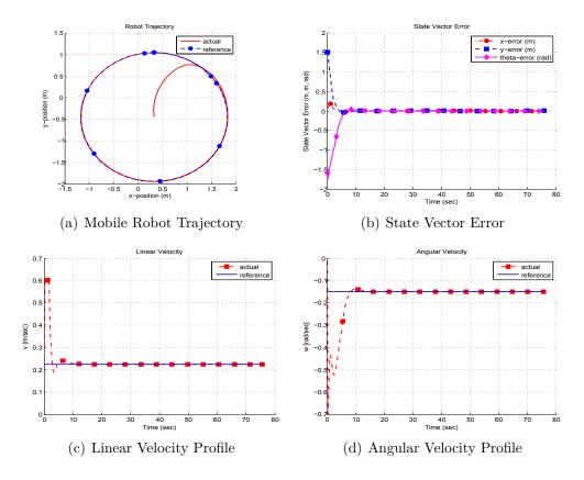
Figure 5.4: Simulation(ACADO) results of trajectory tracking for indoor navigation based on tracking system
