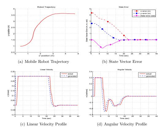
Figure 4.2: Simulation(MobileSim) results of point stabilization for indoor navigation using map based localization
