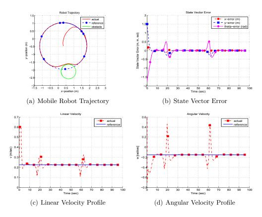
Figure 5.8: Simulation results of trajectory tracking with obstacle avoidance
