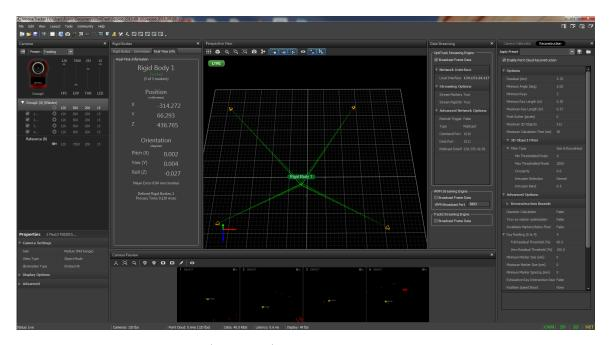
Figure 3.6: Motive (Software) for OptiTrack motion capture system
