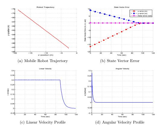
Figure 4.6: Simulation results of point stabilization for outdoor navigation
