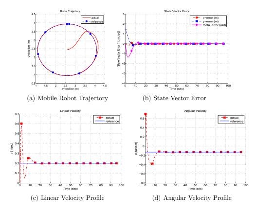
Figure 5.1: Simulation(ACADO) results of trajectory tracking for indoor navigation using map based localization
