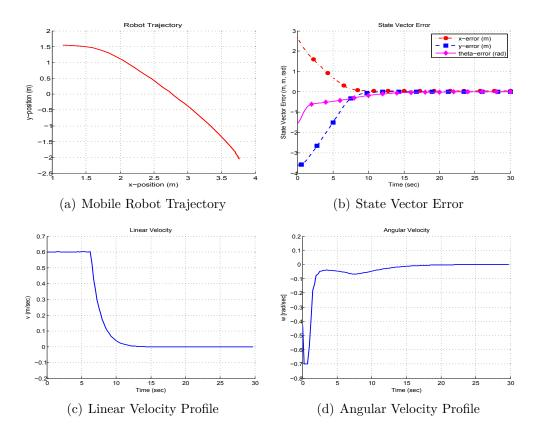
Figure 4.4: Simulation results of point stabilization for indoor navigation using tracking system
