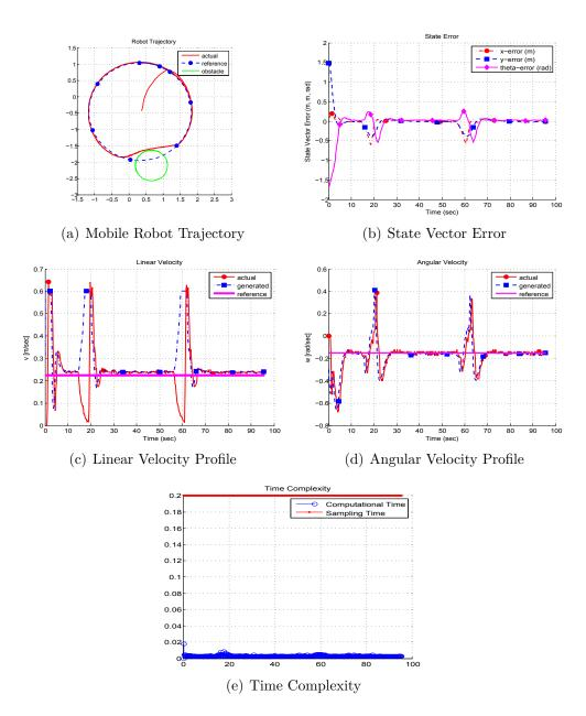
Figure 5.9: Realtime Experimental results of trajectory tracking for obstacle avoidance
