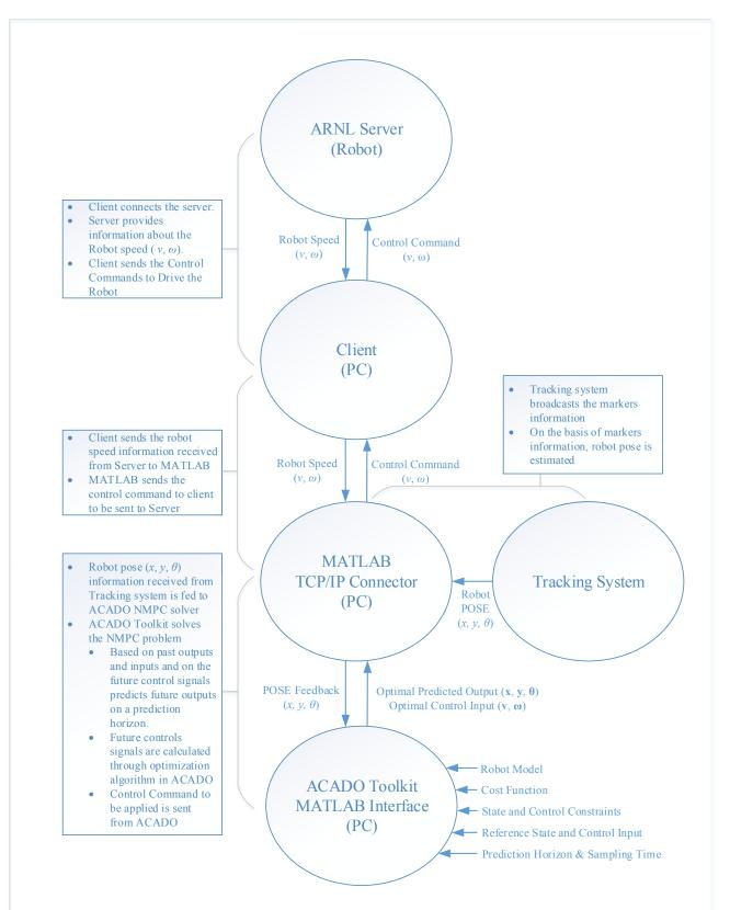
Figure 3.5: Overall Control Strategy for Indoor Navigation using tracking
