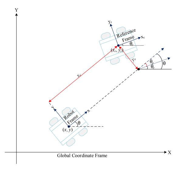
Figure 3.1: Mobile robot in global coordinate frame
