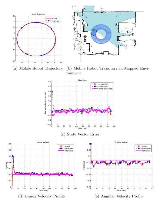
Figure 5.2: Simulation(MobileSim) results of trajectory tracking for indoor navigation using map based localization
