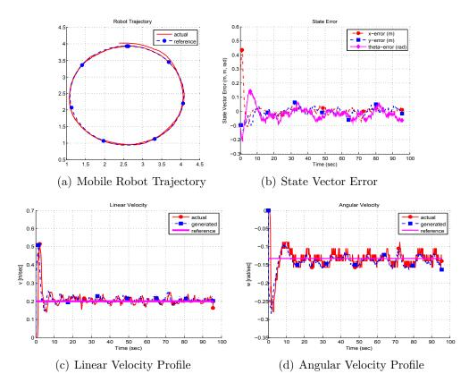
Figure 5.3: Realtime Experimental results of trajectory tracking for indoor navigation using map based localization
