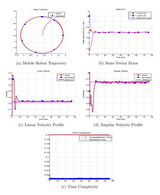
Figure 5.5: Realtime Experimental results of trajectory tracking for indoor navigation based on tracking system
