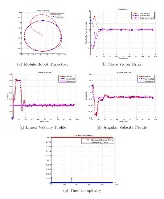
Figure 5.7: Realtime Experimental results of trajectory tracking for outdoor navigation
