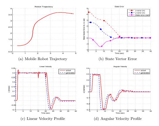
Figure 4.3: Realtime Experimental results of point stabilization for indoor navigation using map based localization
