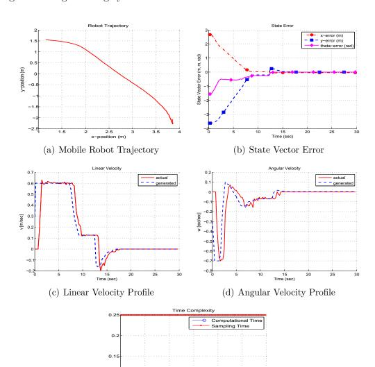
Figure 4.5 shows the real time experimental results run on Seekur Jr. for indoor navigation using tracking system.
