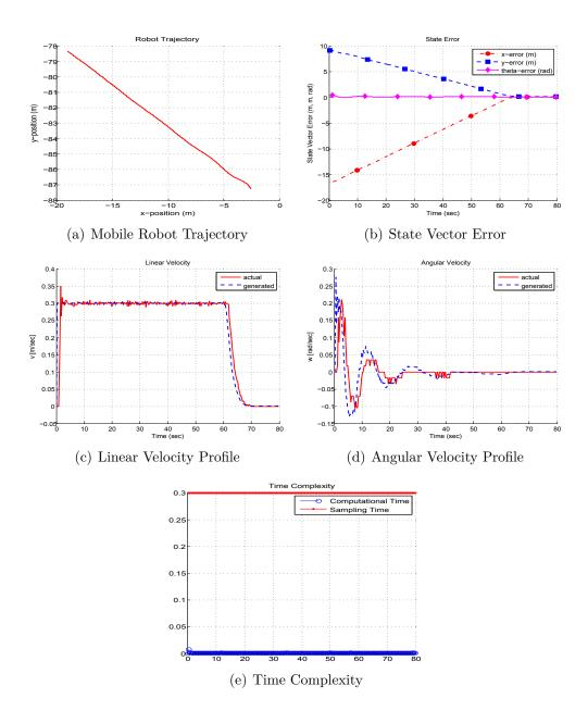
Figure 4.7: Realtime Experimental results of point stabilization for outdoor navigation
