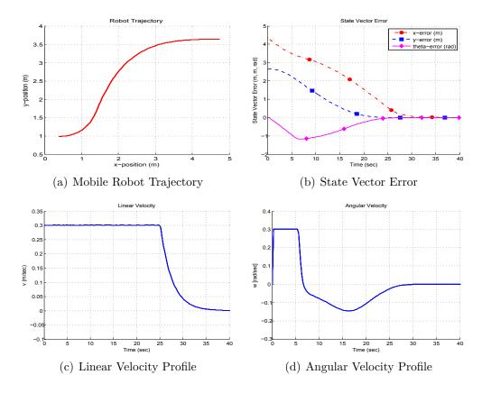
Figure 4.1: Simulation(ACADO) results of point stabilization for indoor navigation using map based localization
