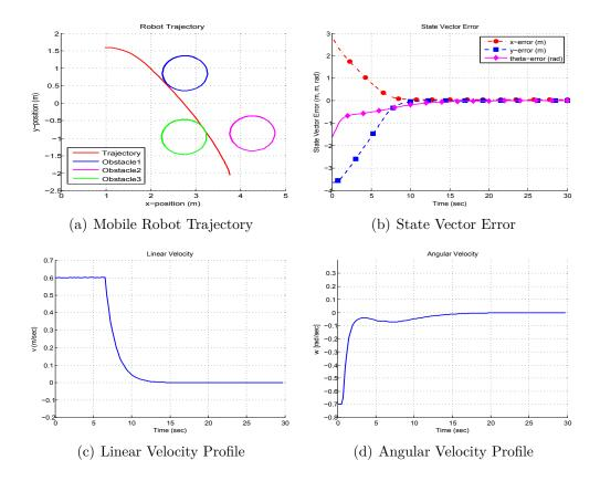
Figure 4.8: Simulation results of point stabilization with obstacle avoidance
