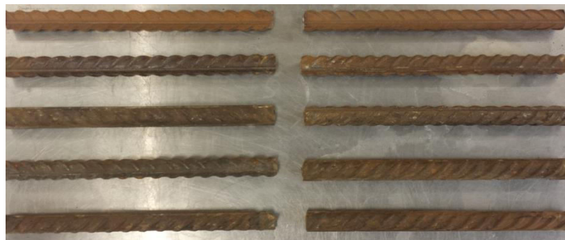
Figure 4.7 Effects of different levels of mass loss in 20 mm cover samples
