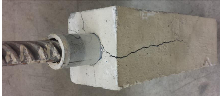
Figure 6.1 Typical bond splitting cracks at failure (example sample: 20M30B0-1)
