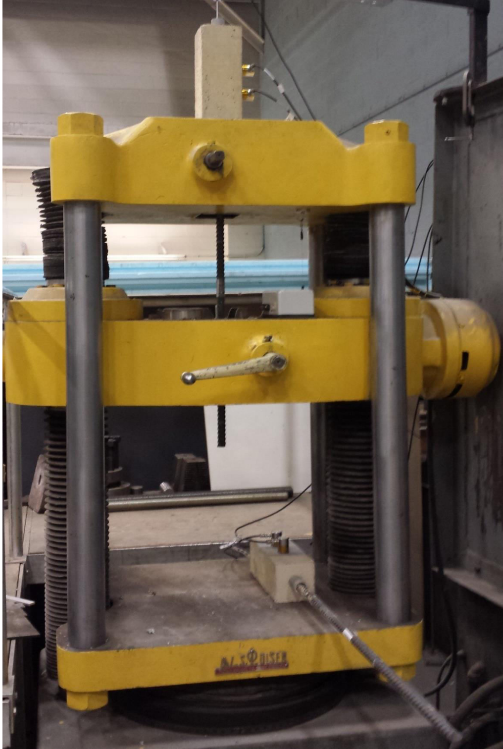
Figure 3.4 Pull-out test and AE monitoring setup: (a) schematic and (b) picture of typical experiment
