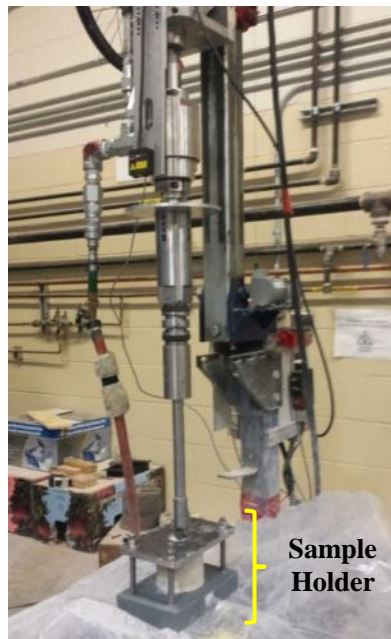
Figure B.1. Lab scale drill rig and sample holder.
