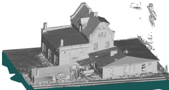
Figure 15. Meshed surface of the building, generated from UAV images, solely. A precise, homogeneous and complete reconstruction could be achieved with the well distributed images of our flight planning and execution concept.
