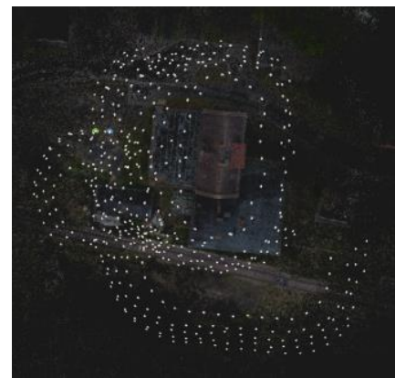
Figure 14: Bird's eye view of the sparse reconstruction (RealityCapture) of the building depicted in Figure 2. Here, the image acquisition was planned and executed using the described software tools.
