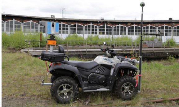
Figure 1. An off-road capable quad, equipped with a variety of sensors, is the core of terrestrial data acquisition and serves as a mobile workstation.
