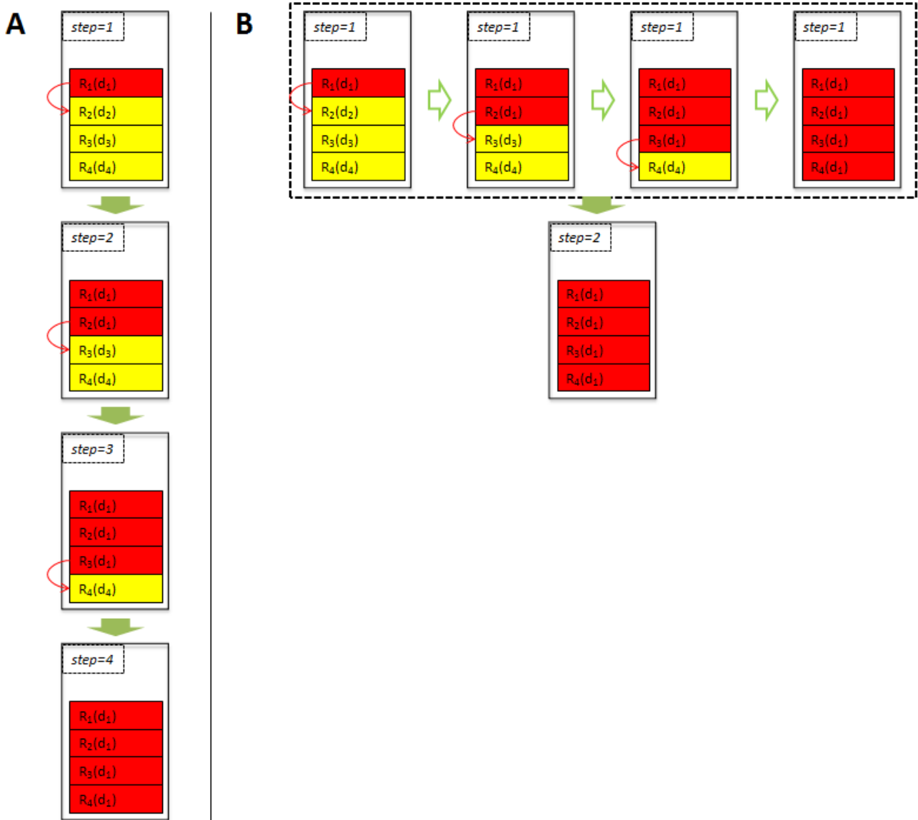
Figure 6.1. Comparison of traditional context-sensitive L-systems and fast information transfer. Using traditional context-sensitive L-systems, a sub-module R_n checks the current state of parameter values in its neighbouring R_{n-1} , therefore the information can only be passed through one sub-module at most after a simulation step. Using fast information transfer, the information can be passed through the whole string after a step regardless how many sub-modules the string has.
