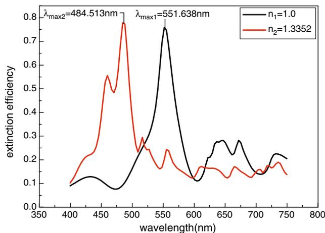
**Fig. 2** FDTD solution calculated result when the refractive index medium surrounding this hybrid nanoparticles are 1.0 and 1.3352, respectively
