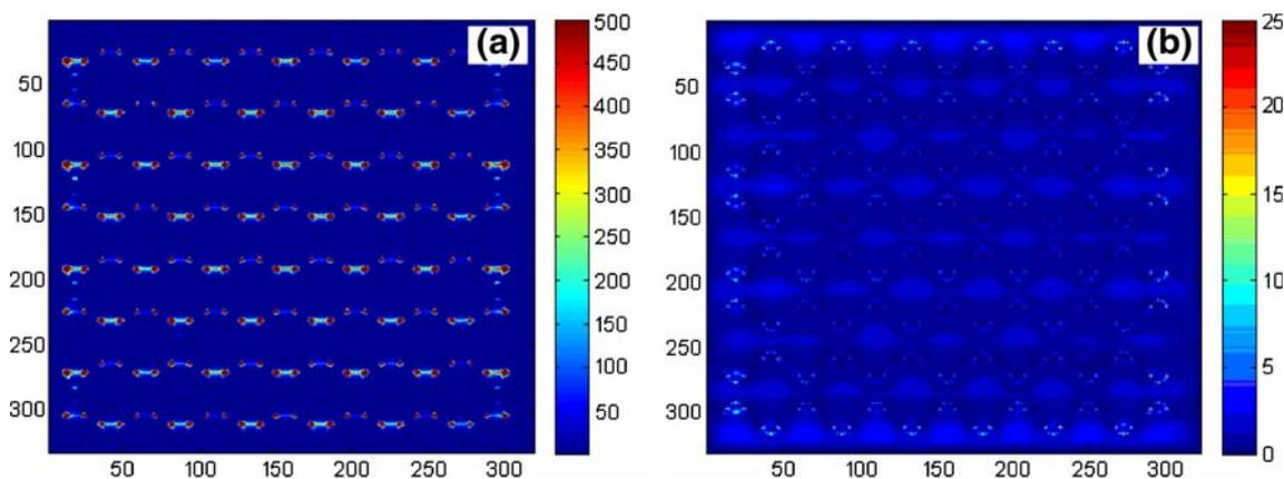
**Fig. 3** FDTD solution calculated electric field result when the incidence light wavelength is equal to the LSPR wavelength. **(a)** Total electric field  $E^2 = E_x^2 + E_y^2 + E_z^2$  from Au surface 5 nm;  $n=$
