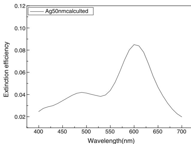
**Fig. 8** Simulation result of extinction efficiency for silver-only nanoparticles. All the parameters are same as the hybrid Au–Ag nanoparticles. Out-of plane height of the silver nanoparticles is 50 nm, and the in plane widths of each nanoparticles is 100 nm. The period of the nanoparticle array is 400 nm and wavelength of the incidence white light source is ranging from 400 nm to 700 nm. The incidence light beam is projected in perpendicular to the substrate simulation
