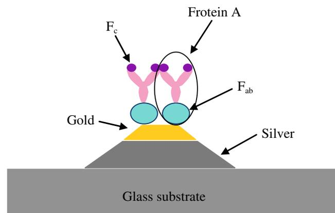
**Fig. 5** Schematic diagram of the Fc directed method binding to the surface of gold nanoparticles
