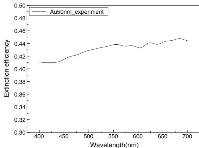
**Fig. 10** Experiment result of extinction efficiency for gold-only nanoparticles
