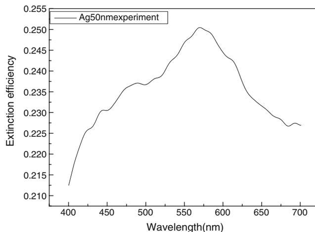
**Fig. 9** Experiment result of extinction efficiency for silver-only nanoparticles
