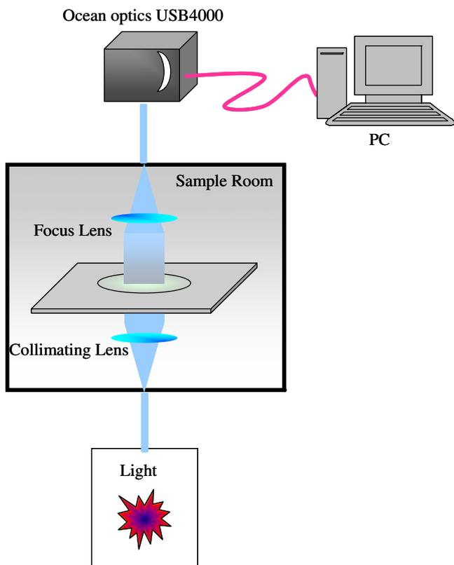
**Fig. 4** A schematic diagram of the light path and measurement set-up of Optical fiber (Ocean Optics USB4000) coupled spectrometric system
