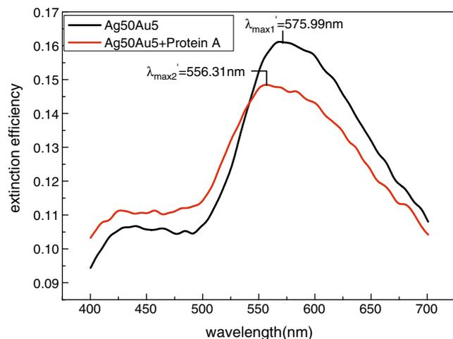
**Fig. 7** Measured spectra for both pure hybrid Au–Ag (thickness of the Ag and Au is 50 nm and 5 nm, respectively) nanoparticles array and binding with protein A
