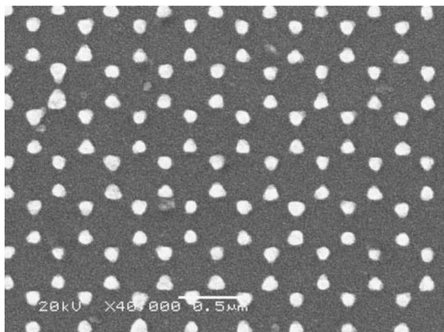
**Fig. 6** SEM image of topography of the triangular hybrid Au–Ag nanoparticles fabricated by NSL
