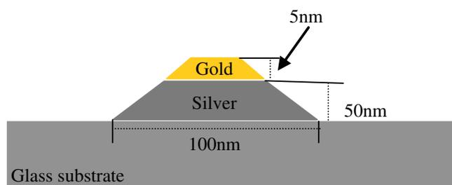
**Fig. 1** Cross-section of a single hybrid Au–Ag triangular nanoparticles
