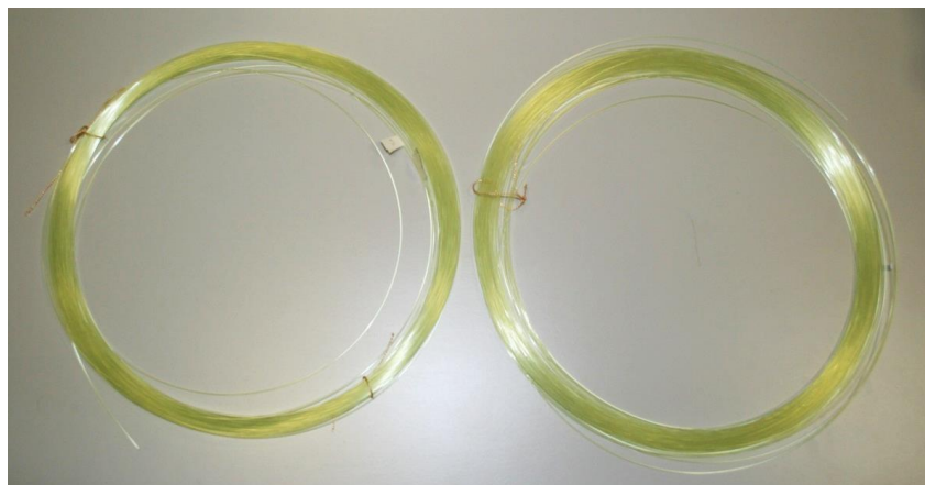
Figure 48: PMMA fluorescent optical fiber (FOF) with 35 ppm of 61d .
