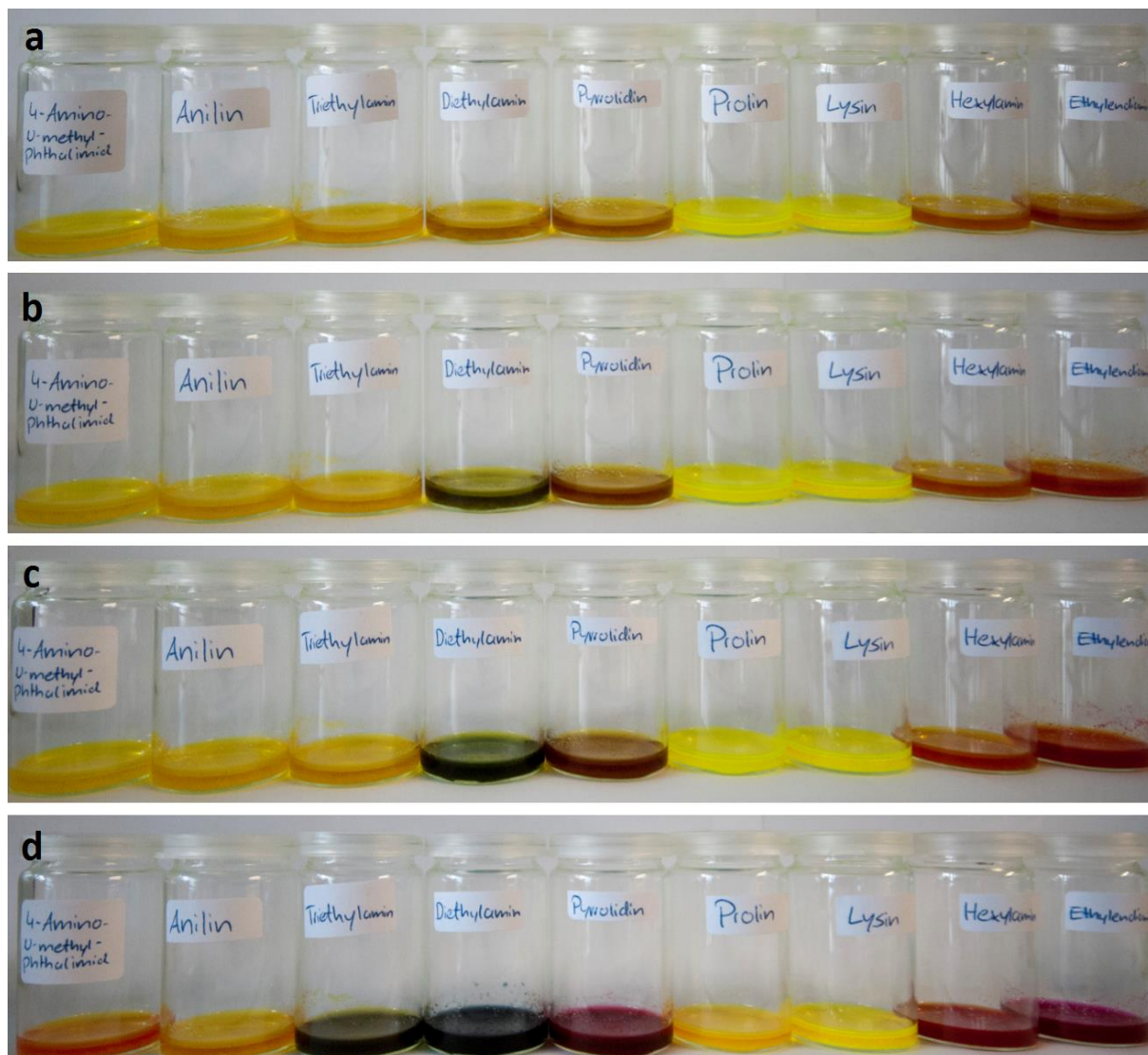
Figure 16: Reaction of N -(tridecan-7-yl)anthracene dicarboximide ( 40 ) in 0.1 M DMF with selected amines after different reaction times at room temperature. From top to bottom: a) Directly after addition; b) after 1 h; c) after 4 h; d) after 1 week. From left to right: 4-Amino- N -methylphthalimid, aniline, triethylamine, diethylamine, pyrrolidine, ( S )-proline, ( S )-lysine, 1-hexylamine, 1,2-diaminoethane.
