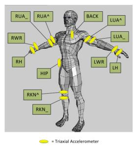
Figure 7.1: accelerometer placement for OPP dataset
