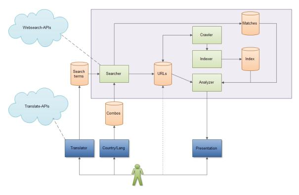
Figure 4.3: System structure
