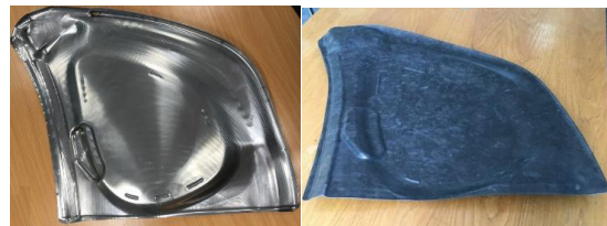
Fig. 2. Incremental Sheet Forming tool skin and molded component from HiLiTe material
