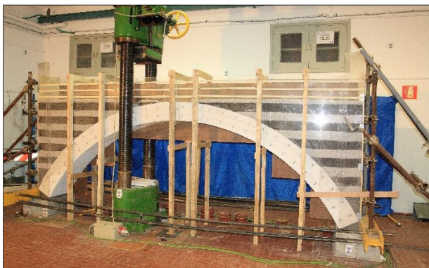
Figure 3. The arch model.
