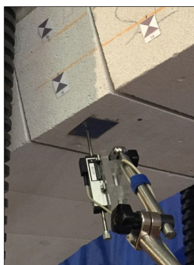
Figure 8. A detail of LVDT.
